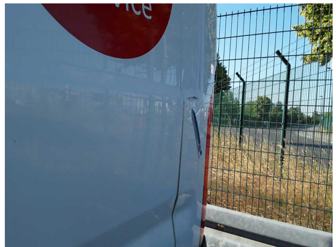
Damage 8: Side panel - rear left side: Side panel (Eckteil) - Dent / paintcoat damage - Repair and paint
