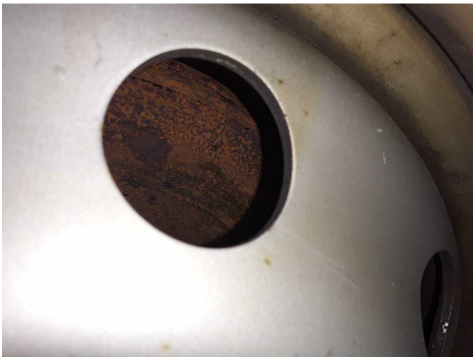
Damage 7: Braking system: Brake discs and brake pads - front - Corrosion - Replace
