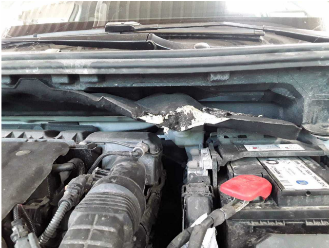
Damage 2: Cab: Insulation lining - Damaged - Replace
