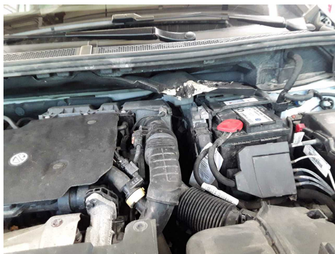
Damage 2: Cab: Insulation lining - Damaged - Replace
