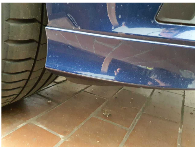
Damage 2: Front bumper: Spoiler - Scratch(es) - Smart repair
