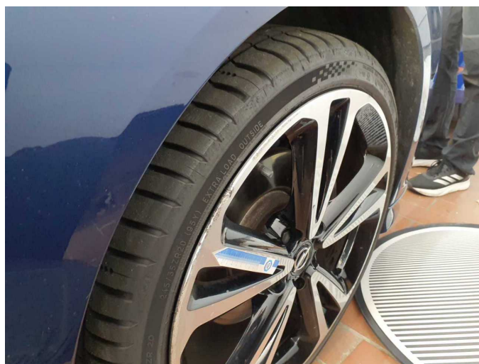
Damage 5: Wheel / tyres: Alloy rim - front right side (Sicherheitsrelevant) - Scratched - Replace
