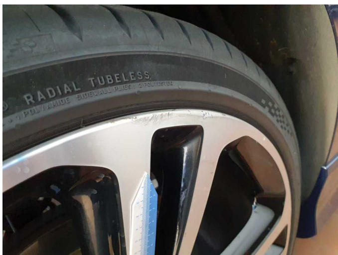
Damage 4: Wheel / tyres: Alloy rim - rear right side - Unprofessionally repaired - Replace
