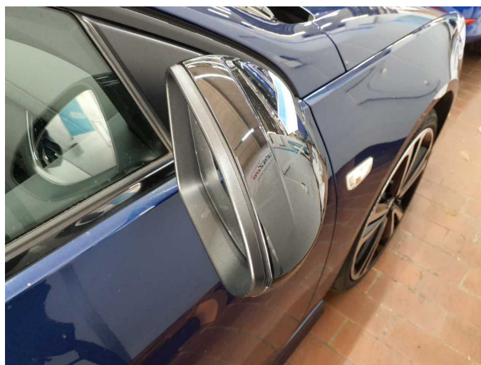
Damage 1: Wing mirror - right side: Cap - Scratch(es) - Smart repair
