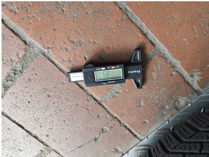
Damage 3: 2nd wheel set: 2 tyres - Worn - Replace
