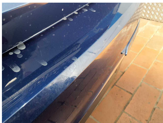
Damage 6: Rear bumper: Rear bumper - Scratch(es) - Paint
