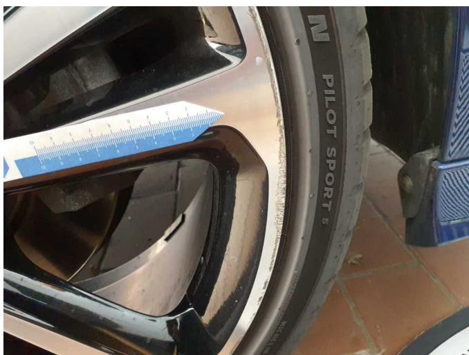
Damage 5: Wheel / tyres: Alloy rim - front right side (Sicherheitsrelevant) - Scratched - Replace
