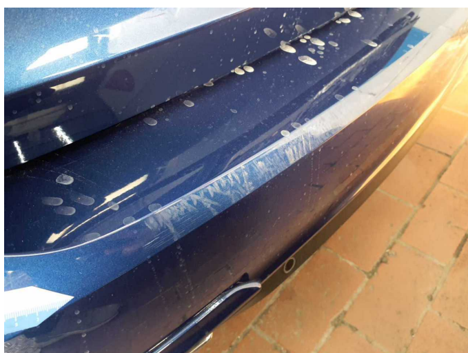
Damage 6: Rear bumper: Rear bumper - Scratch(es) - Paint
