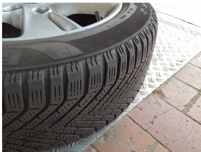
Damage 3: 2nd wheel set: 2 tyres - Worn - Replace
