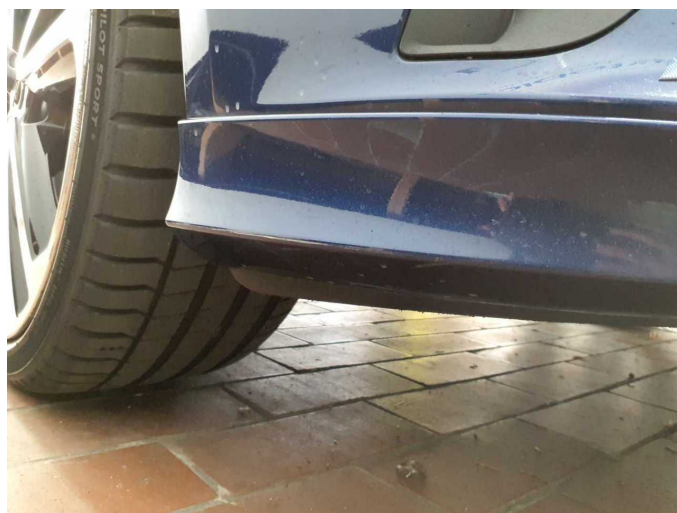
Damage 2: Front bumper: Spoiler - Scratch(es) - Smart repair
