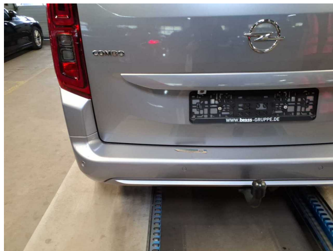
Damage 14: Rear bumper: Rear bumper - Scratched - Paint
