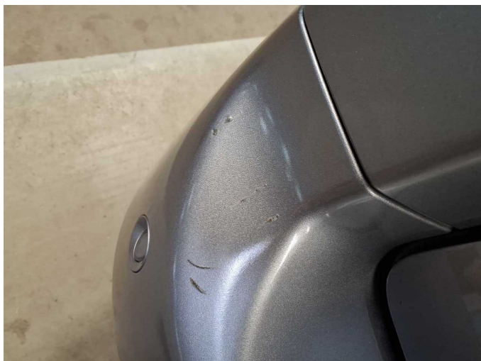
Damage 14: Rear bumper: Rear bumper - Scratched - Paint
