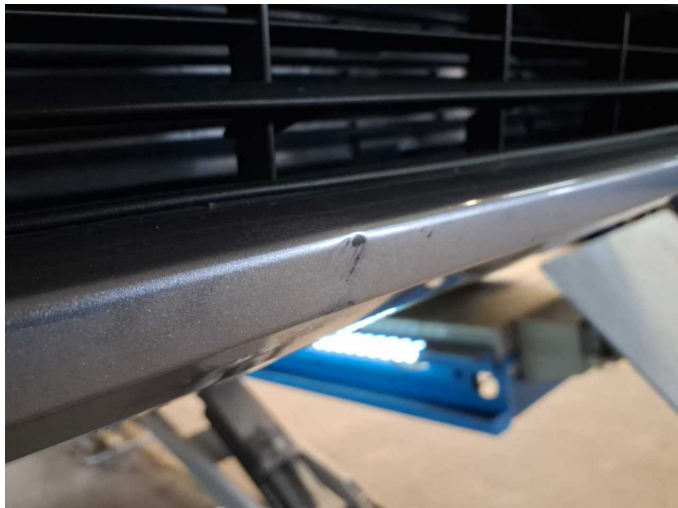
Damage 8: Front bumper: Spoiler - Scratch(es) - Smart repair
