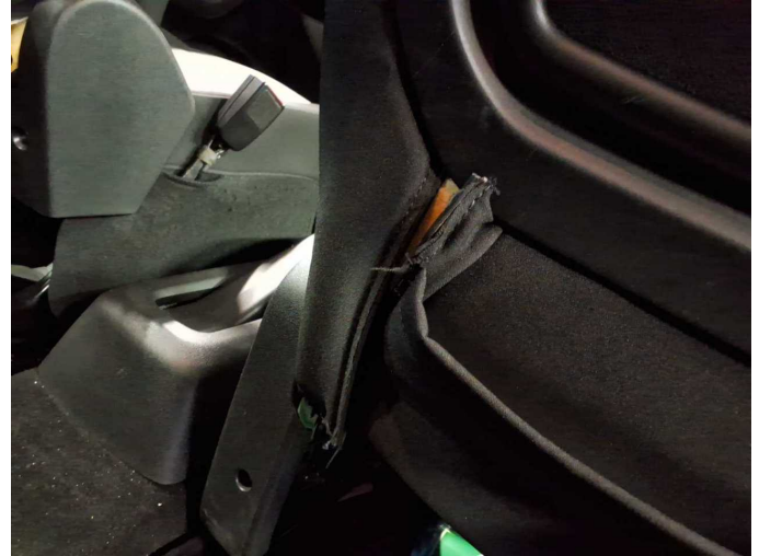
Damage 17: Seat - front: Backrest cover - right side - Broken / torn - Replace
