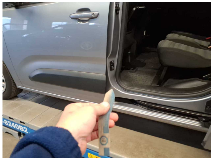
Damage 6: Body: B-pillar - left side - dent(s) - Smooth repair work
