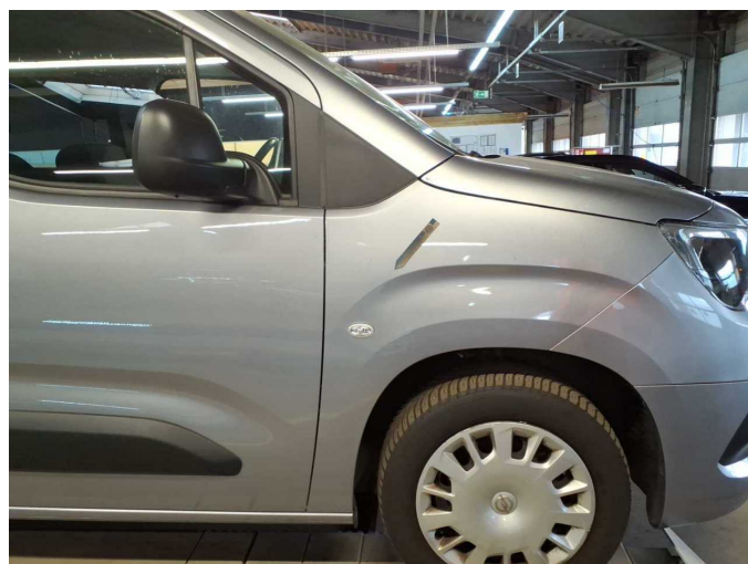
Damage 7: Mudguard - right side: Mudguard - right side - dent(s) - Smooth repair work
