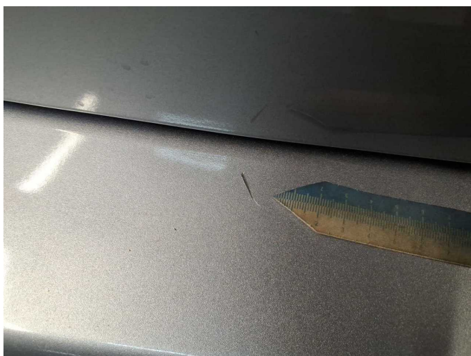
Damage 14: Rear bumper: Rear bumper - Scratched - Paint
