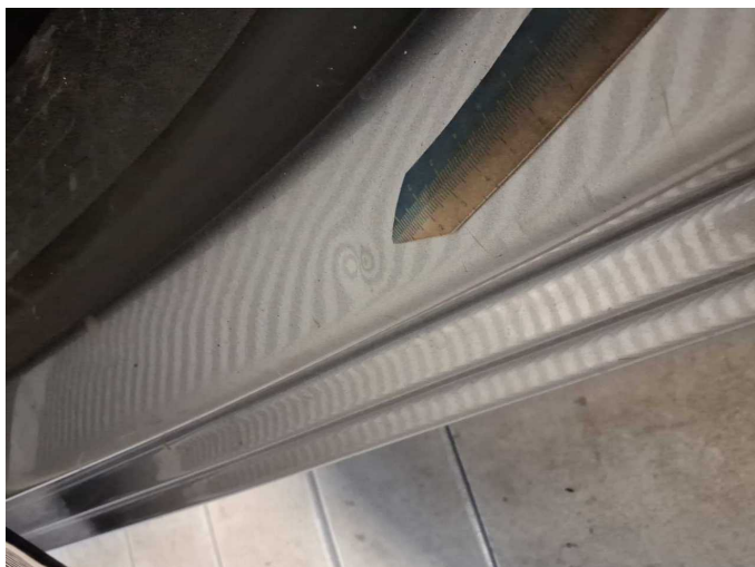
Damage 5: Sill - left side: Sill - dent(s) - Smooth repair work
