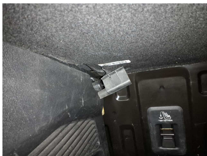
Damage 13: Interior: Rear shelf (Halter) - Broken / torn - Replace
