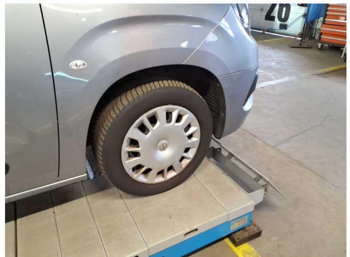
Damage 3: Wheel / tyres: Wheel cover - front right side - Scratched - Replace
