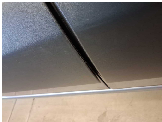
Wear and tear 3: Door - front left side: Brightware - lower - Scratch(es) - No deduction
