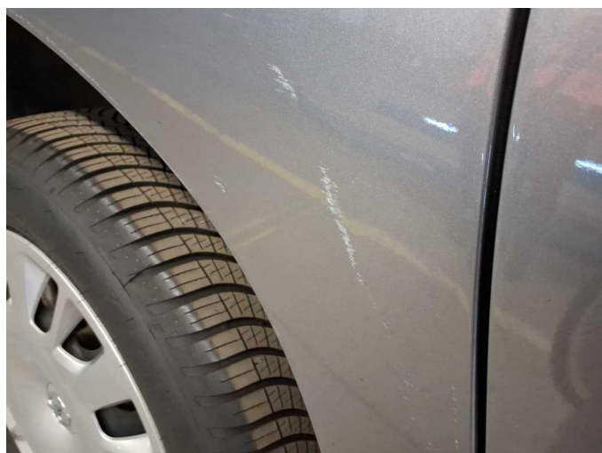
Damage 19: Side panel - rear right side: Side panel (Verkratzt) - Deformed - Repair and paint
