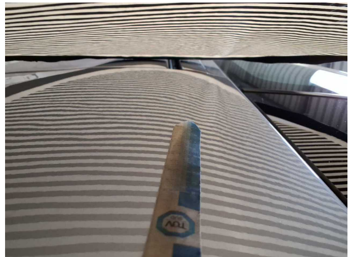
Damage 18: Sliding door, right: Sliding door with glass panel (Wellig, Einschlüsse) - Unprofessionally repaired - Repair and paint
