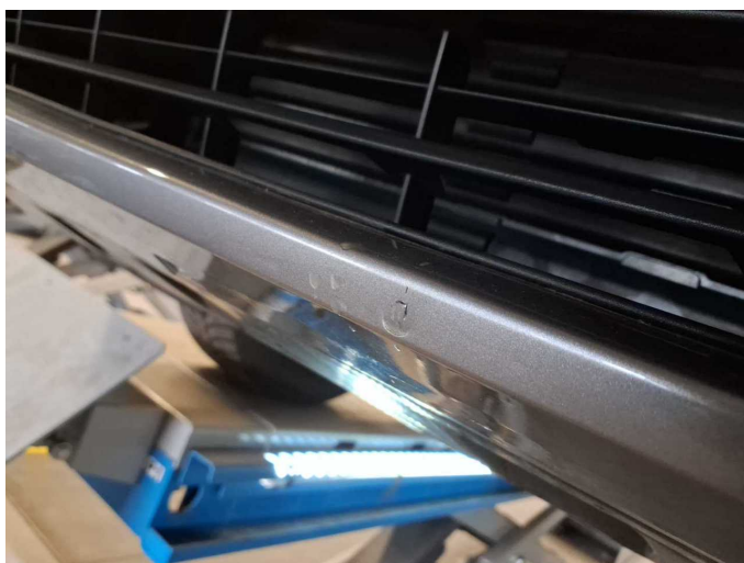
Damage 8: Front bumper: Spoiler - Scratch(es) - Smart repair
