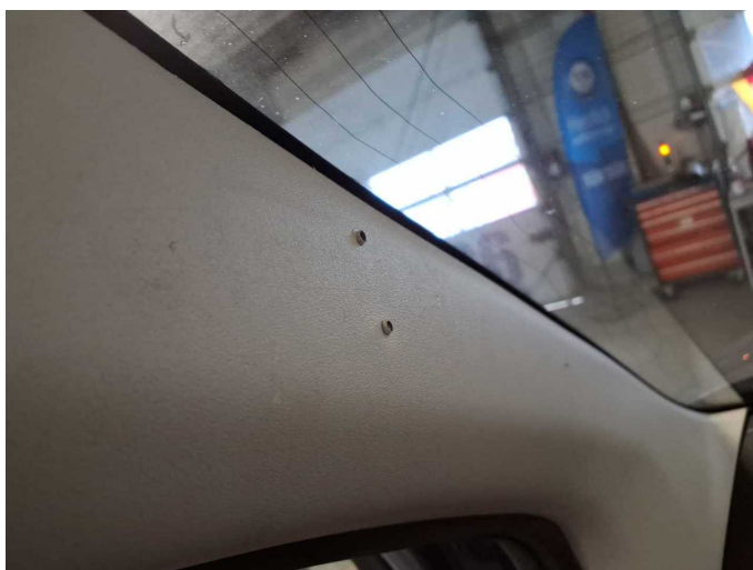
Damage 9: Trim / covers: A-pillar - trim - interior, left side - Holes - Replace
