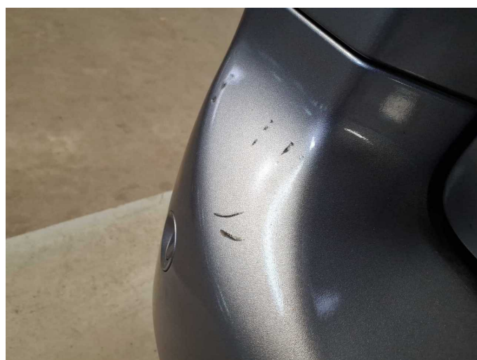
Damage 14: Rear bumper: Rear bumper - Scratched - Paint
