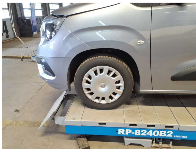
Damage 10: Wheel / tyres: Tyre - front - Does not meet the leasing specifications - Replace
