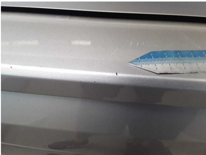
Damage 4: Rear bumper: Rear bumper - Scratch(es) - Paint
