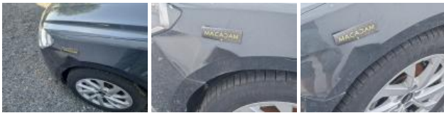
Wing RL, Scratch(es), Spot repair
