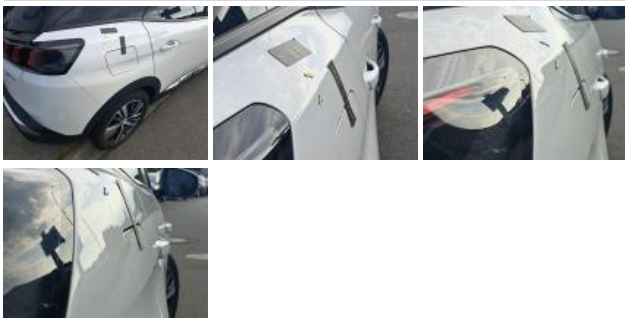
Door FR, Dent(s), Repair and paint (complete)
