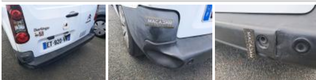
Bumper R, Broken, Replace
