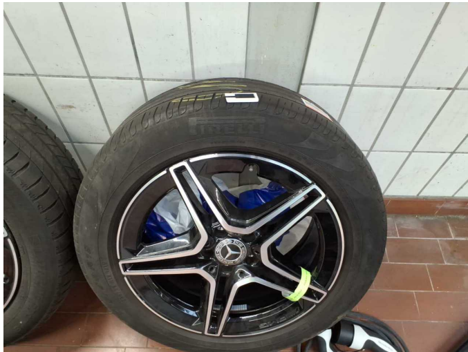
Damage 9: 2nd wheel set: 2 tyres - Worn - Replace
