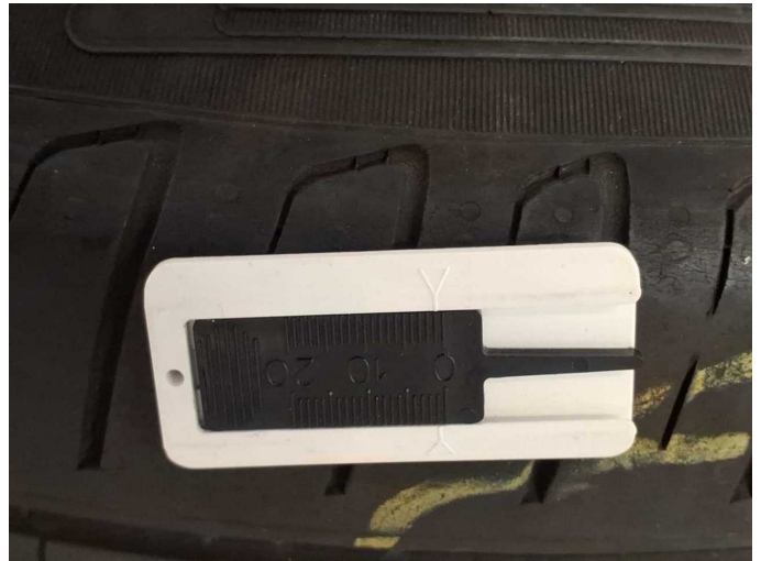
Damage 9: 2nd wheel set: 2 tyres - Worn - Replace
