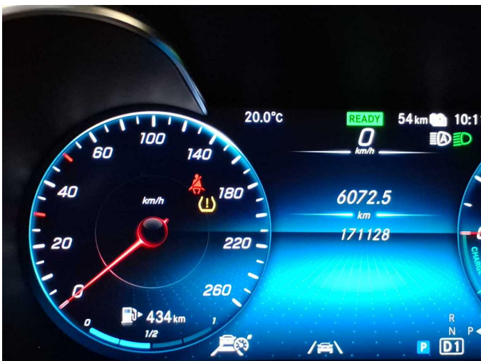
Damage 4: Wheel / tyres: Pressure sensor (Reifendruck) - Electrical fault - Diagnosed and repair if necessary
