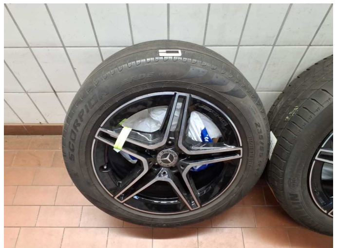
Damage 9: 2nd wheel set: 2 tyres - Worn - Replace
