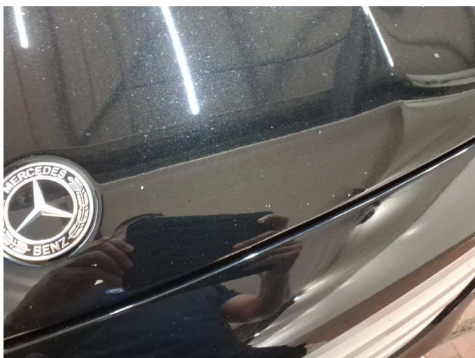
Damage 4: Bonnet: Bonnet - Stone chips - Paint
