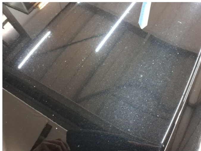
Damage 4: Bonnet: Bonnet - Stone chips - Paint
