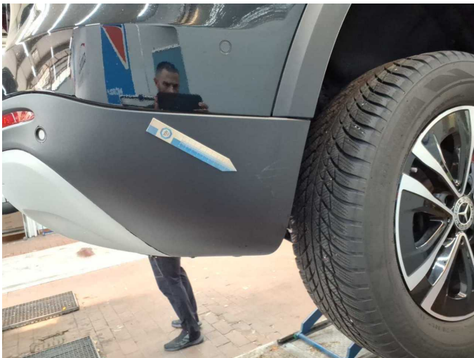
Damage 1: Rear bumper: Spoiler - Scratch(es) - Loss in value
