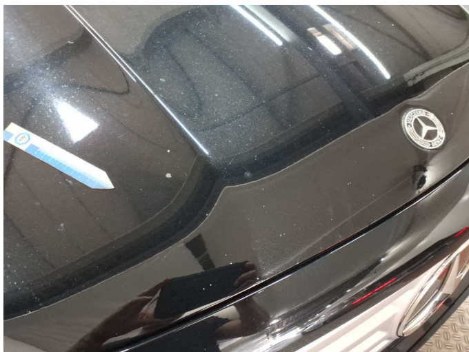
Damage 4: Bonnet: Bonnet - Stone chips - Paint
