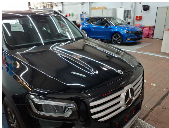
Damage 4: Bonnet: Bonnet - Stone chips - Paint
