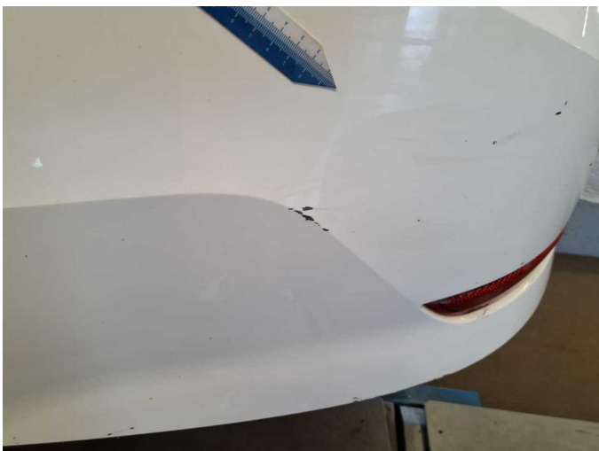
Damage 4: Rear bumper: Rear bumper - Scratch(es) - Repair and paint
