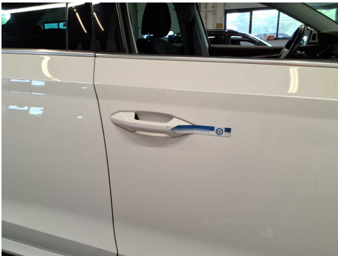
Damage 1: Door - front right side: Door handle - outside - Stone chips - Smart repair
