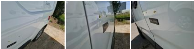
Door trim FL, Deformed / Strained, Replace
