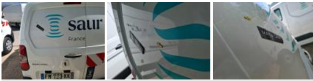
Bumper corner RR, Deformed / Strained, Repair and paint (complete)
