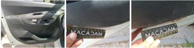
Door FL, Dent(s), Repair and paint (complete)
