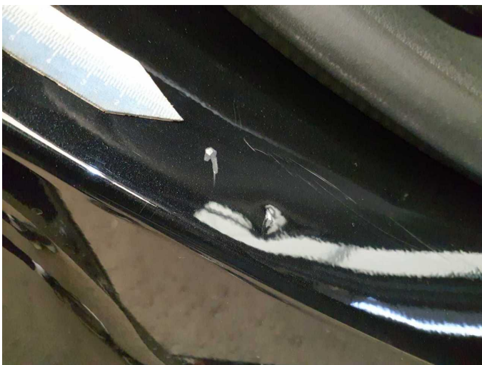
Damage 6: Side panel - rear right side: Sill - Dent / paintcoat damage - Smart repair
