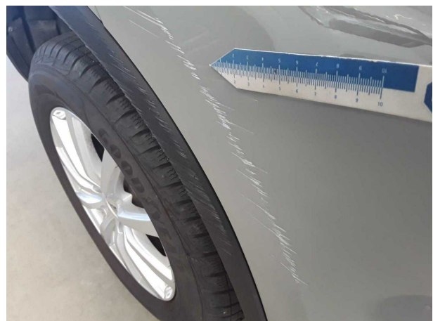
Damage #7: Door - rear right side: Door - Scratched - Repair and paint
