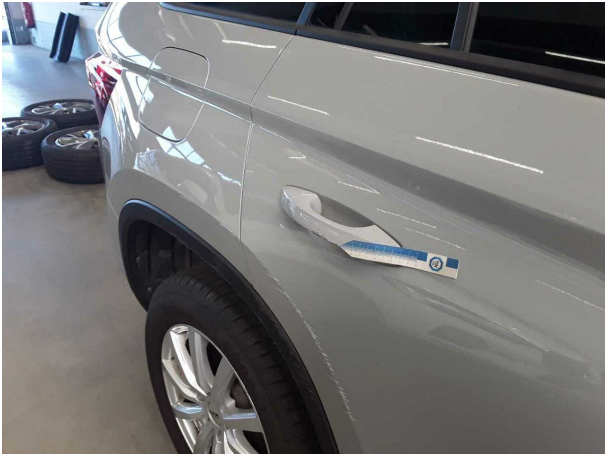
Damage #1: Door - rear right side: Door handle - outside - Scratched - Repair and paint
