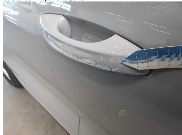
Damage #2: Door - front right side: Door handle - outside - Scratched - Repair and paint
