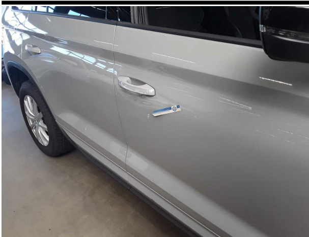
Damage #8: Door - front right side: Door - Dent / paintcoat damage - Repair and paint
