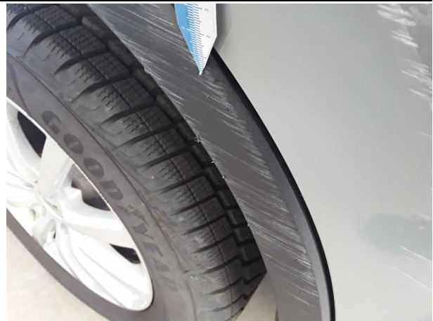
Damage #4: Side panel - rear right side: Wheel well extensio... Scratched - Replace
