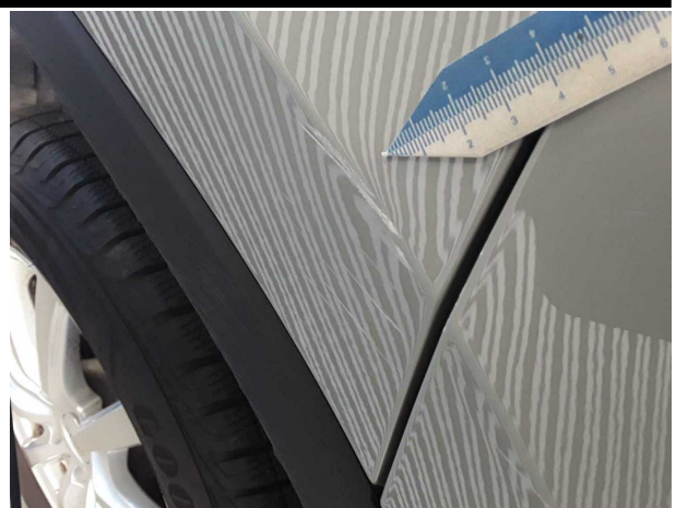
Damage #9: Side panel - rear right side: Side panel - Scratch... - Repair and paint
