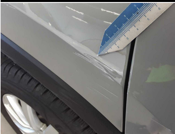
Damage #9: Side panel - rear right side: Side panel - Scratched - Repair and paint
