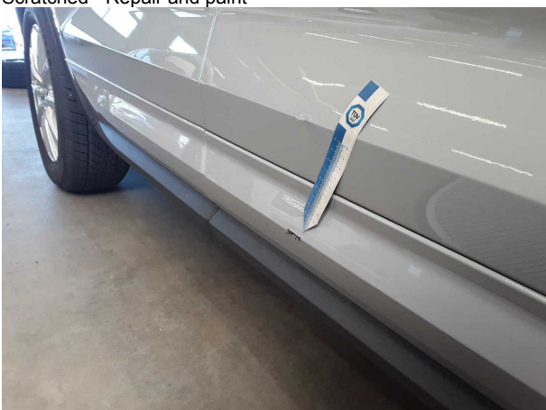
Damage #3: Door - front right side: Brightware - lower - Scratched - Paint
