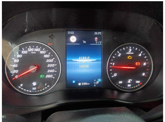
Damage 3: Instrument panel: Indicator light (Motorkontrolle) - on - Perform diagnosis
