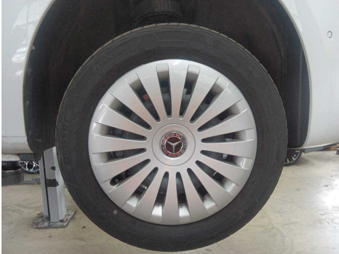
Damage 2: Wheel / tyres: Tyre - front right side (Restlichen 3 Reifen 4,5mm) - Worn - Replace
