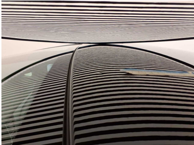
Damage 9: Roof: Roof - dent(s) - Smooth repair work
