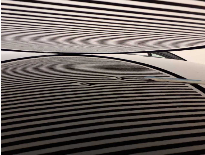
Damage 9: Roof: Roof - dent(s) - Smooth repair work
