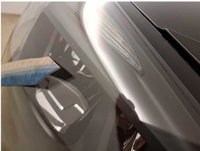
Damage 11: Headlight: Headlight - right side - Scratch(es) - Replace
