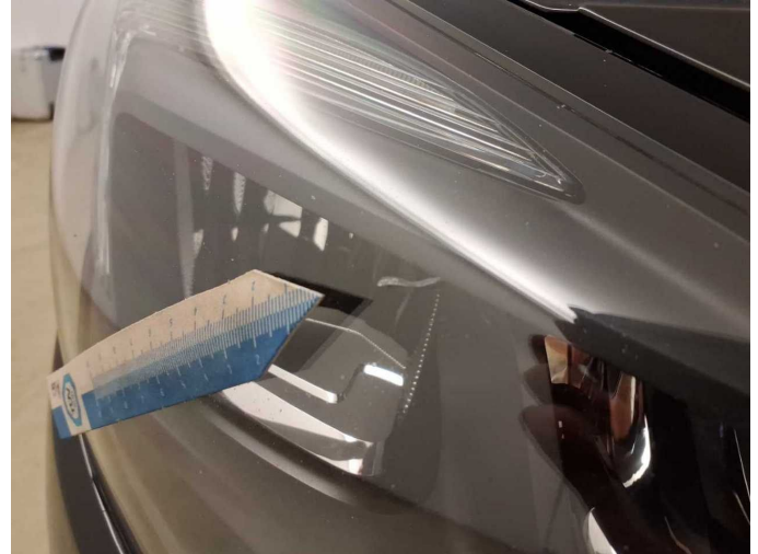
Damage 11: Headlight: Headlight - right side - Scratch(es) - Replace
