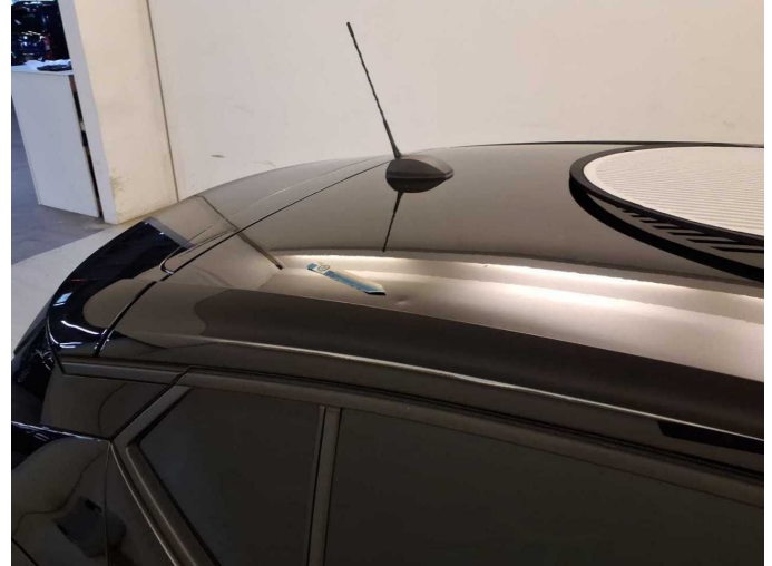
Damage 9: Roof: Roof - dent(s) - Smooth repair work
