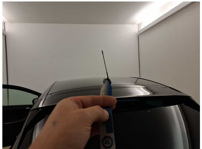
Damage 3: Roof: Stub aerial - Broken / torn - Replace
