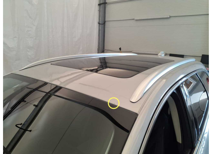
Damage 1: Roof: Roof - Stone chips - Smart repair
