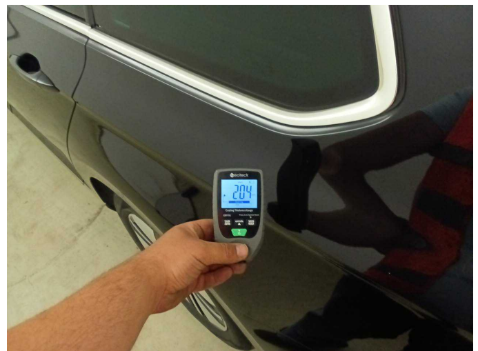
Side panel - rear left side: 204 µm
