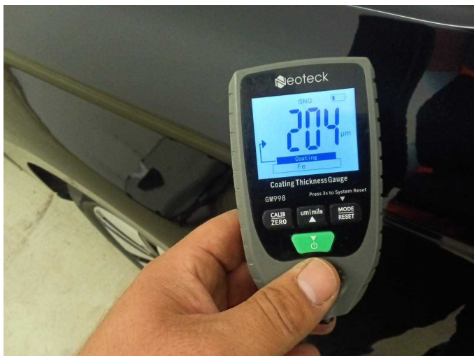
Side panel - rear left side: 204 µm
