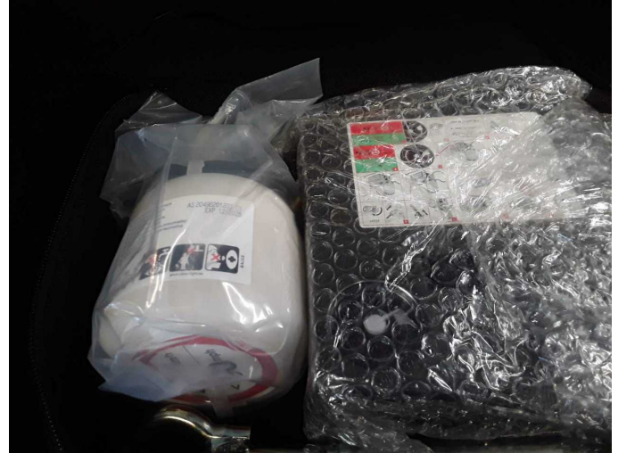
Damage 2: Equipment: Tirefit filler - Expired - Replace
