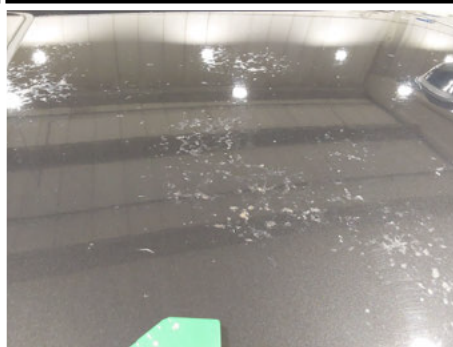
Roof / - / Paint etching
