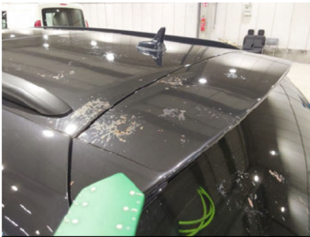
Tailgate / Boot door / - / Paint etching
