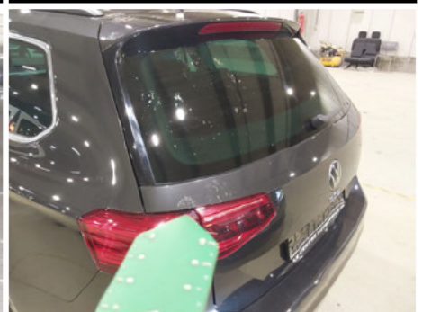
Tailgate / Boot door / - / Paint etching
