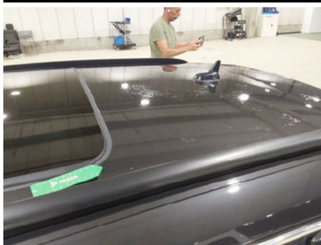
Roof / - / Paint etching
