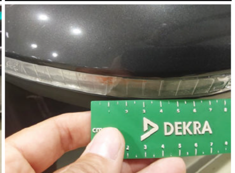
Side turning sign signal / Front Left / Broken
