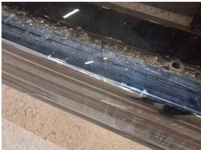
Damage 3: Rear bumper: Rear bumper - Scratch(es) - Paint
