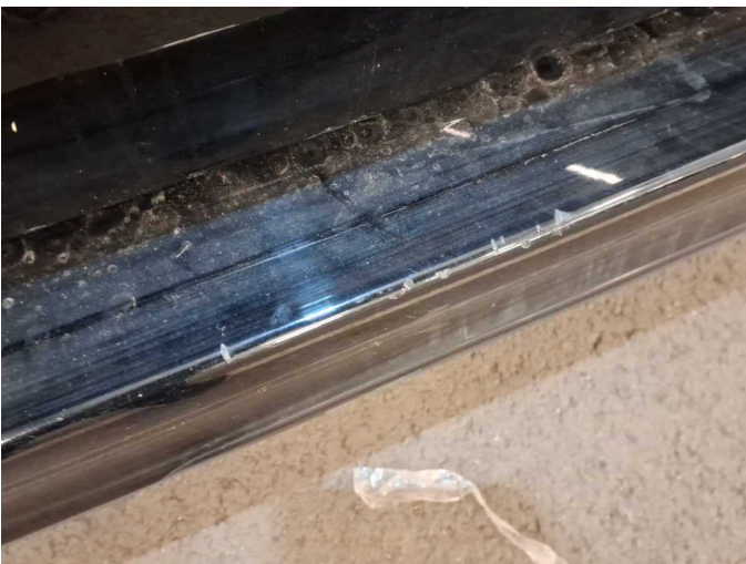
Damage 3: Rear bumper: Rear bumper - Scratch(es) - Paint
