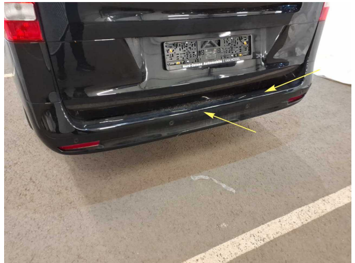
Damage 3: Rear bumper: Rear bumper - Scratch(es) - Paint
