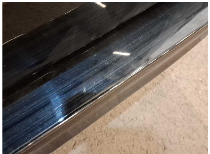
Damage 3: Rear bumper: Rear bumper - Scratch(es) - Paint
