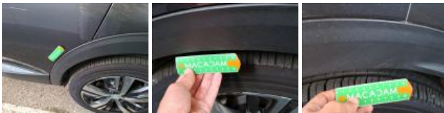
Wing trim RL, Scratch(es), Replace
