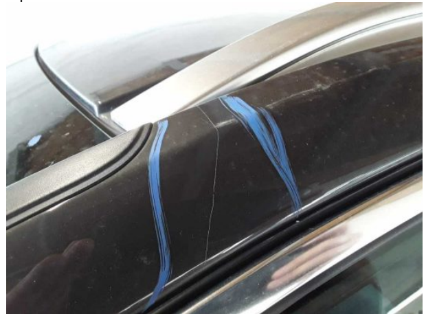
Damage #6: Roof: Roof rail - left side - Scratched - Paint
