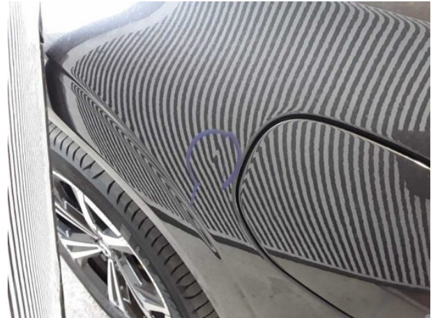
Damage #2: Mudguard - left side: Mudguard - left side - dent(...) - Smooth repair work
