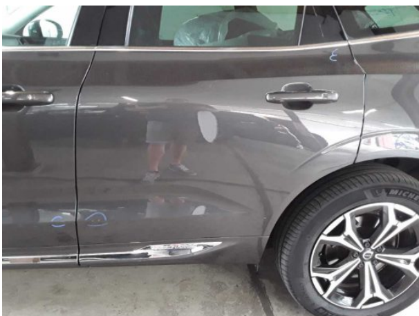
Damage #7: Door - rear left side: Door - Scratched - Paint
