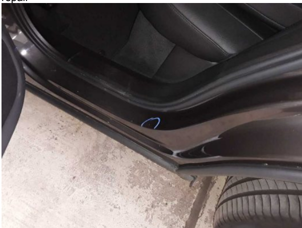
Damage #4: Side panel - rear left side: Sill - Scratched - Smart repair
