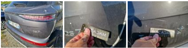
Fog light RL, Broken, Replace
