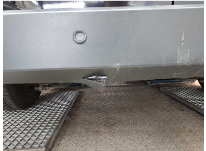
Damage 3: Rear bumper: Rear bumper - Broken / torn - Replace
