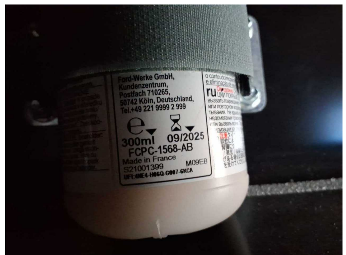
Damage 2: Equipment: Tirefit filler - Expired - Replace
