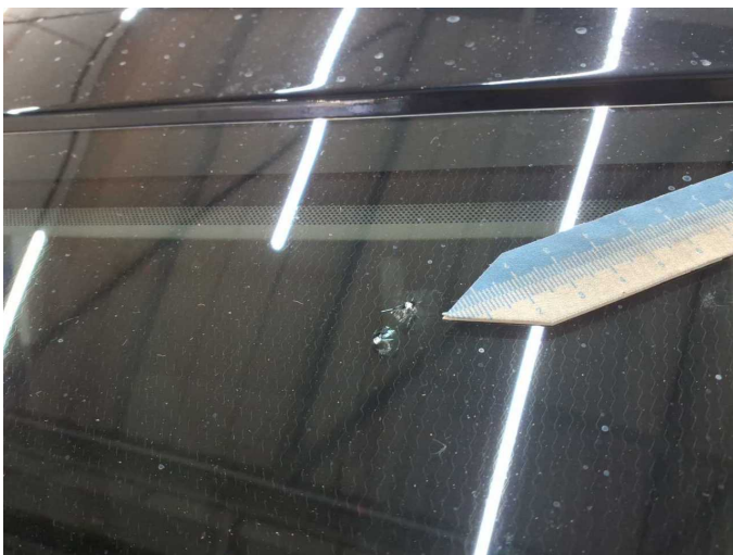
Damage 4: Vehicle glazing: Windscreen - Stone chips - repair according to calculation
