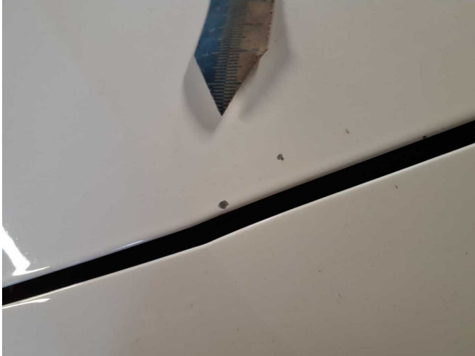
Damage 13: Bonnet: Bonnet - Stone chips - Paint
