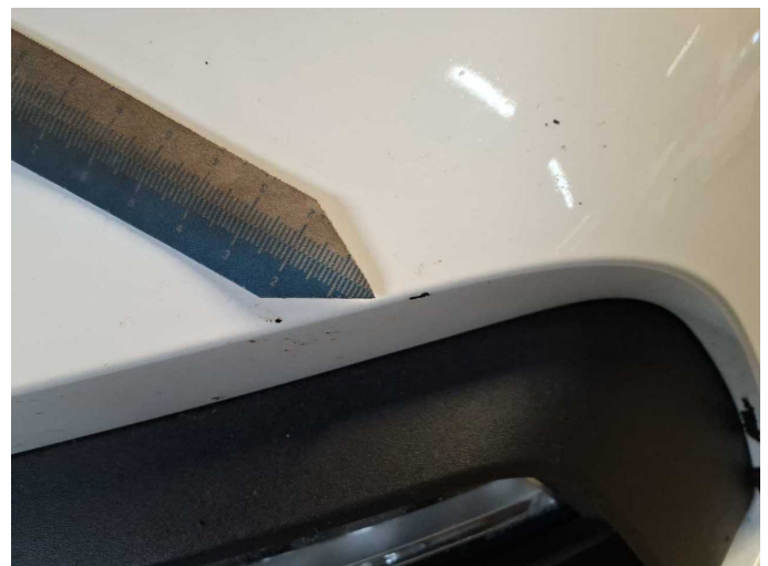
Damage 14: Front bumper: Front bumper - Scratched - Paint
