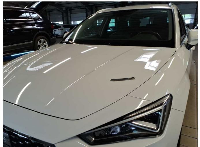
Damage 13: Bonnet: Bonnet - Stone chips - Paint
