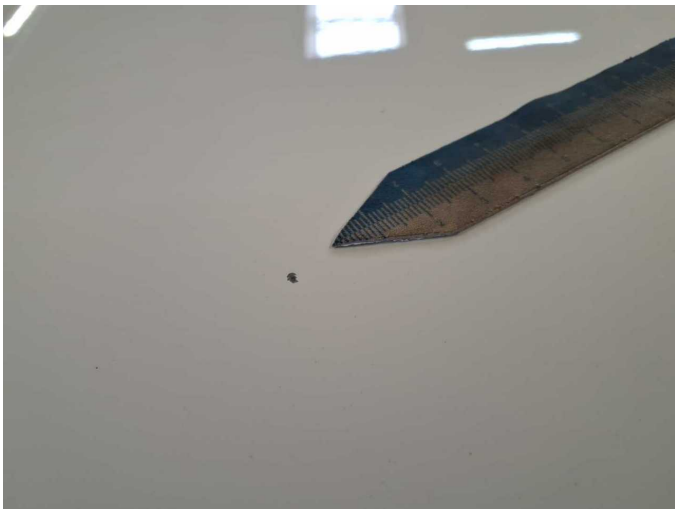
Damage 13: Bonnet: Bonnet - Stone chips - Paint
