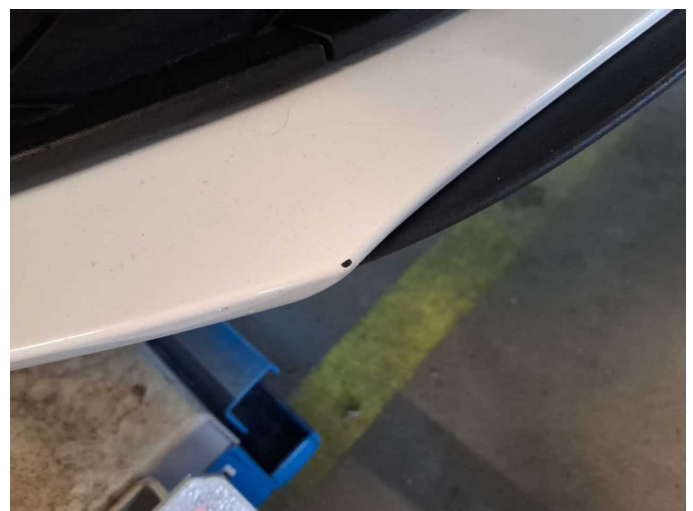
Damage 14: Front bumper: Front bumper - Scratched - Paint
