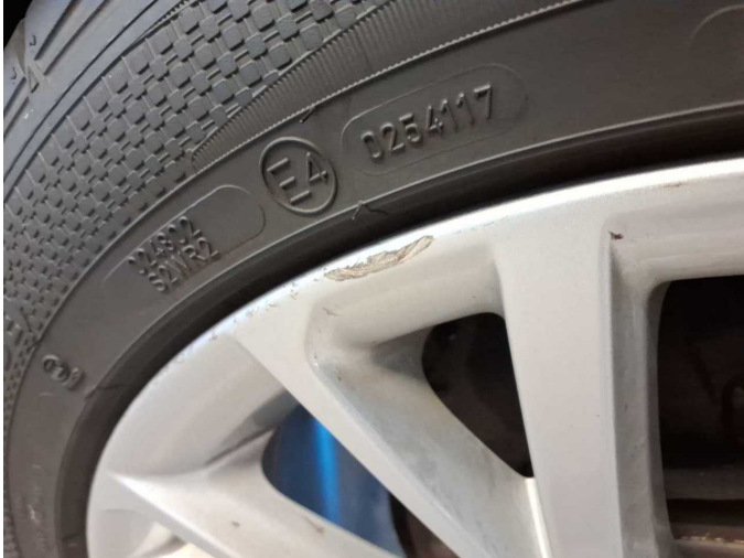
Damage 10: Wheel / tyres: Alloy rim - rear left side - Scratched - Loss in value
