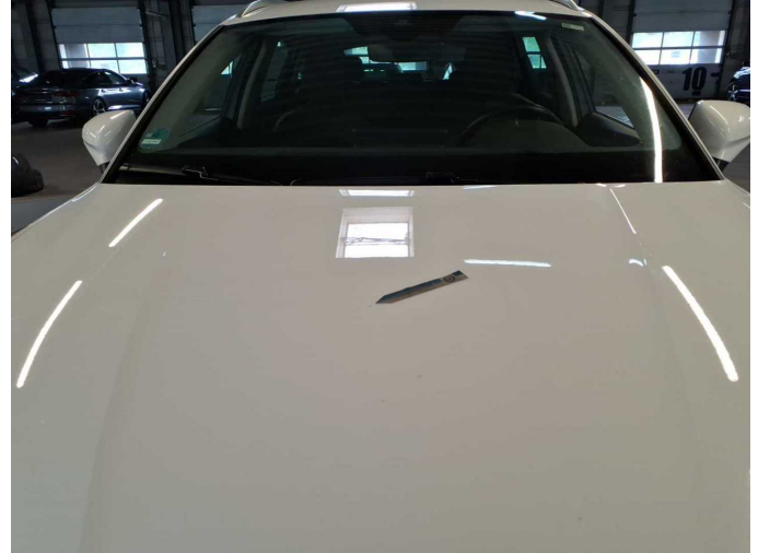
Damage 13: Bonnet: Bonnet - Stone chips - Paint
