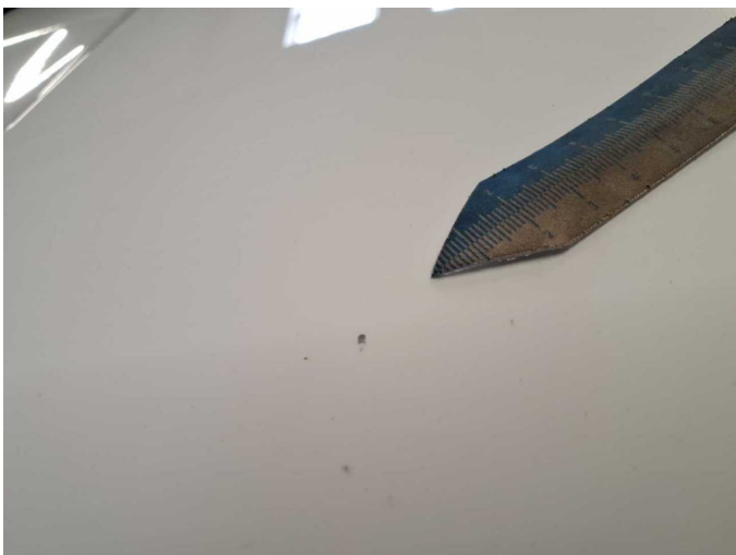
Damage 13: Bonnet: Bonnet - Stone chips - Paint
