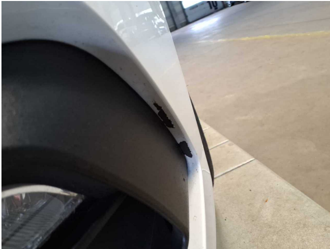
Damage 14: Front bumper: Front bumper - Scratched - Paint
