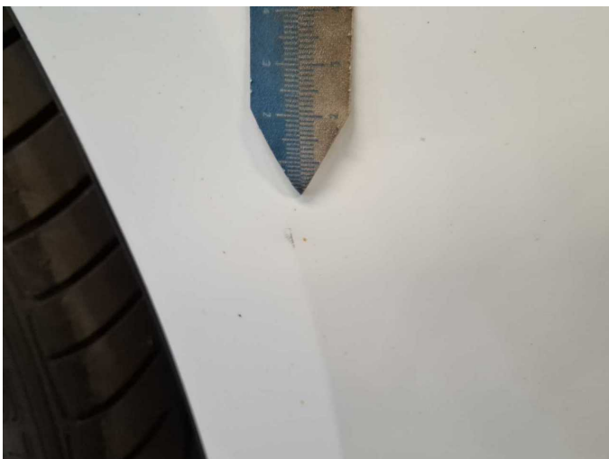
Damage 7: Mudguard - left side: Mudguard - left side - Dent / paintcoat damage - Smart repair
