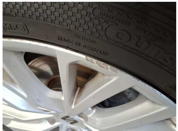
Damage 11: Wheel / tyres: Alloy rim - front right side - Scratch(es) - Loss in value
