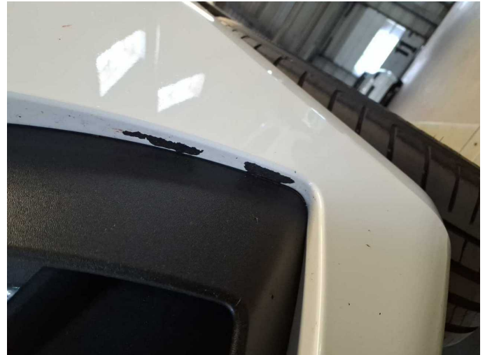
Damage 14: Front bumper: Front bumper - Scratched - Paint
