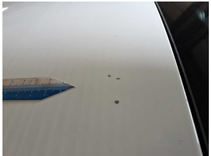
Damage 15: Roof: Roof - Stone chips - Paint
