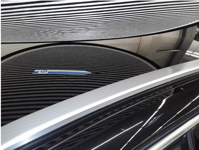
Damage 3: Roof: Roof - dent(s) - Smart repair
