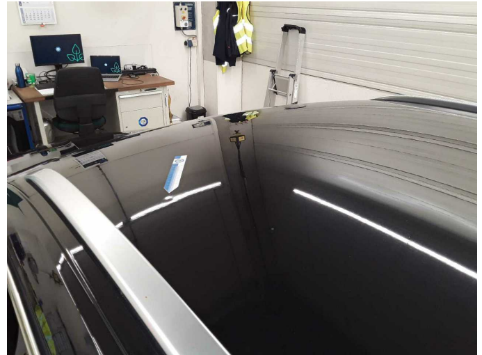
Damage 3: Roof: Roof - dent(s) - Smart repair
