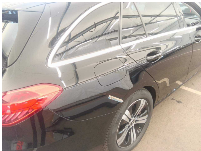
Damage 2: Side panel - rear right side: Mudguard - rear right side - Scratch(es) - Smart repair
