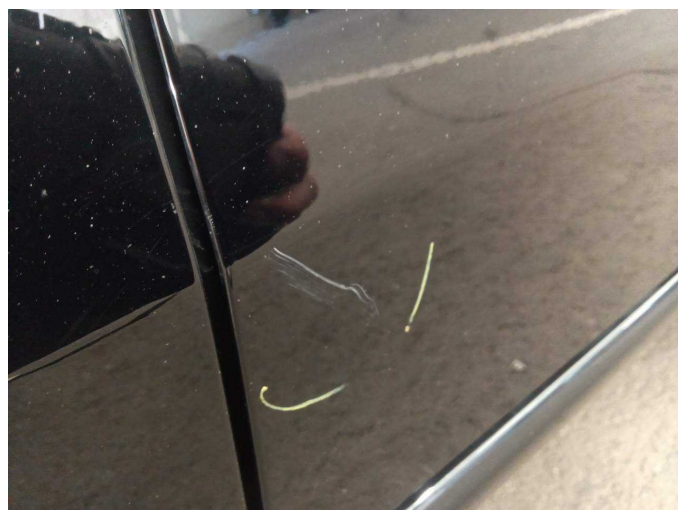
Damage 4: Mudguard - right side: Mudguard - right side - Scratch(es) - Paint
