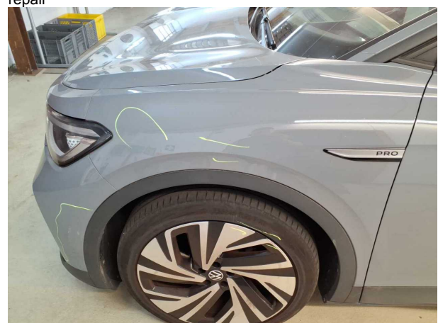
Damage #11: Mudguard - left side: Mudguard - left side - Scratched - Repair and paint
