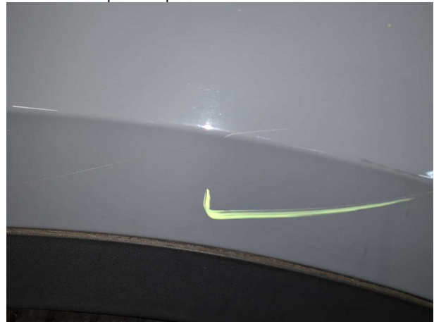
Damage #12: Mudguard - right side: Mudguard - right side - Scratch(es) - Repair and paint
