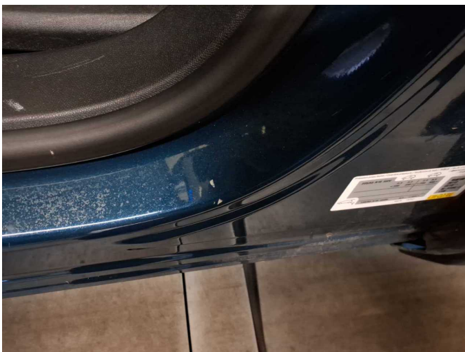
Damage 4: Body: B-pillar - left side - Scratch(es) - Smart repair
