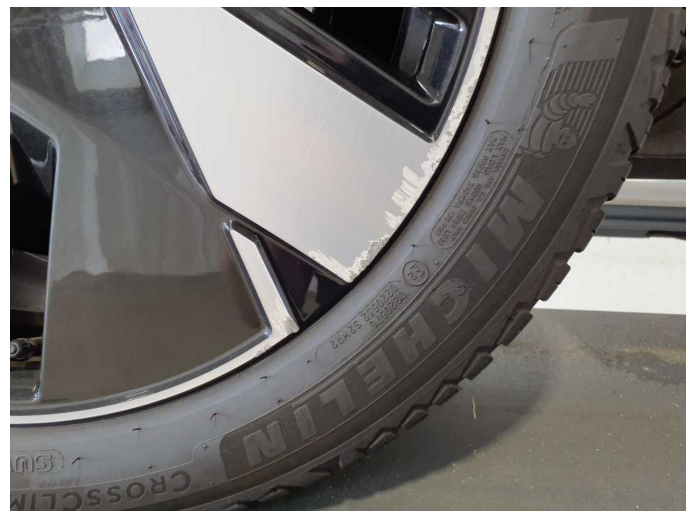
Damage 4: Wheel / tyres: Alloy rim - rear right side - Scratch(es) - Replace
