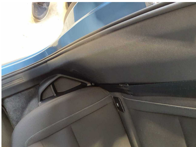
Damage 2: Side panel - rear right side: Interior trim - Scratch(es) - Replace
