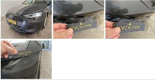
Bonnet, Chemical polution, Repair and paint (complete)
