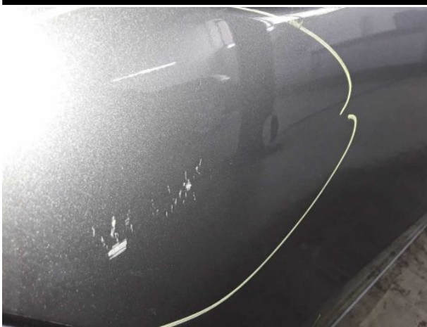
Damage #12: Door - rear right side: Door - Dent / paintcoat dama... - Repair and paint
