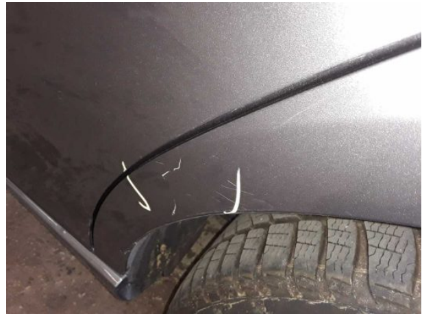
Damage #14: Side panel - rear left side: Side panel - Scratch... - Repair and paint
