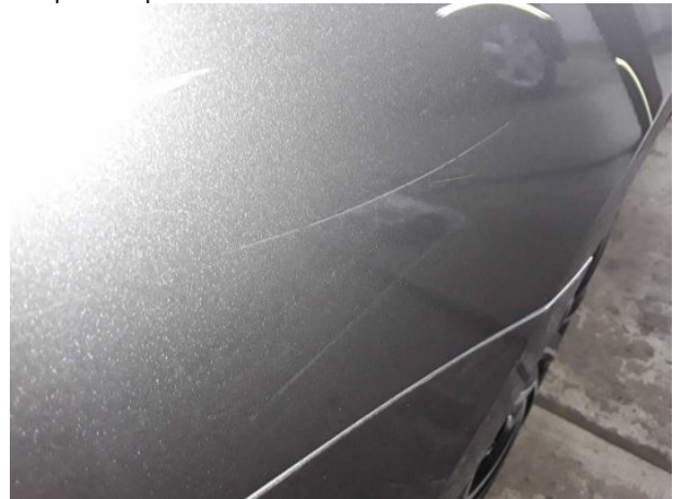
Damage #15: Side panel - rear right side: Side panel - Scratched - Repair and paint
