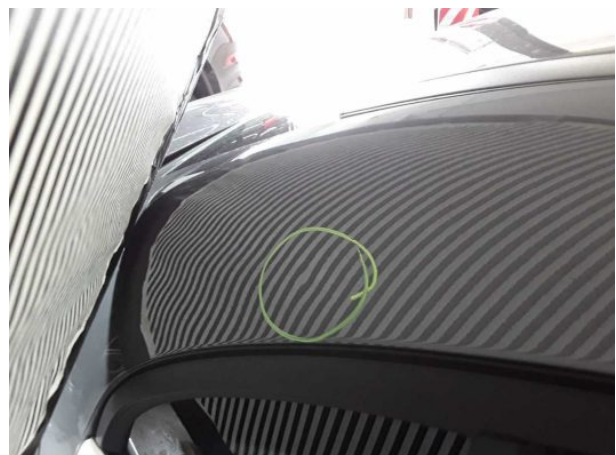
Damage #5: Roof: Roof rail - right side - dent(s) - Smooth repair work
