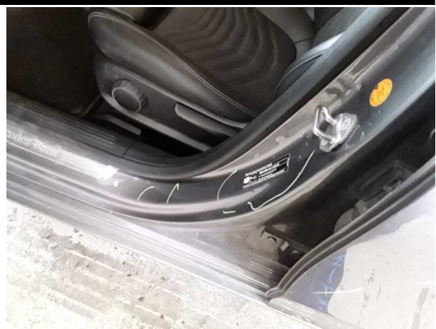
Damage #7: Sill - left side: Sill - Dent / paintcoat damage - Repair and paint
