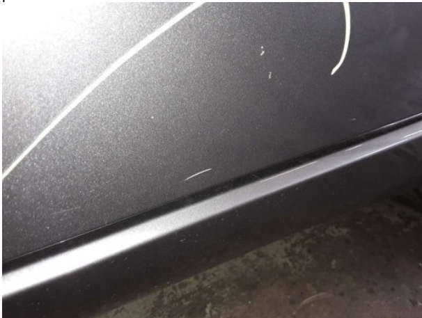
Damage #11: Door - rear left side: Door - Scratched - Repair and paint
