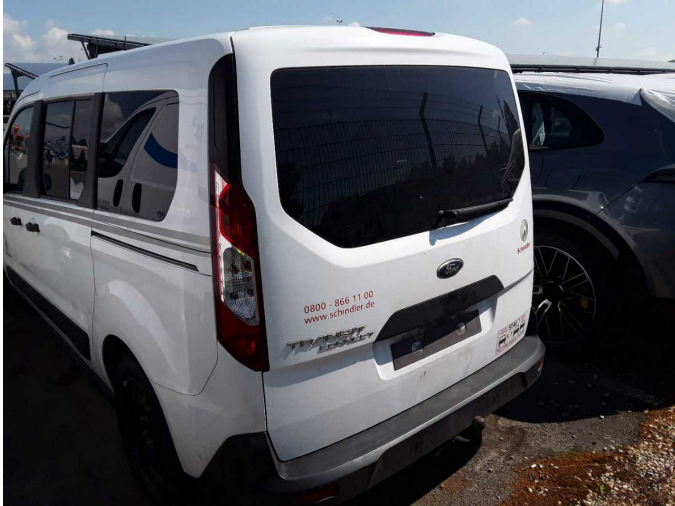
Damage 2: Body: Body - Glued / labelled - De-glue / neutralise
