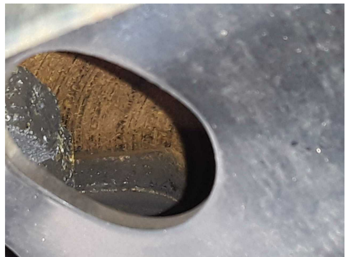
Damage 5: Braking system: Brake discs and brake pads - front (Standsschaden) - Corrosion - Replace
