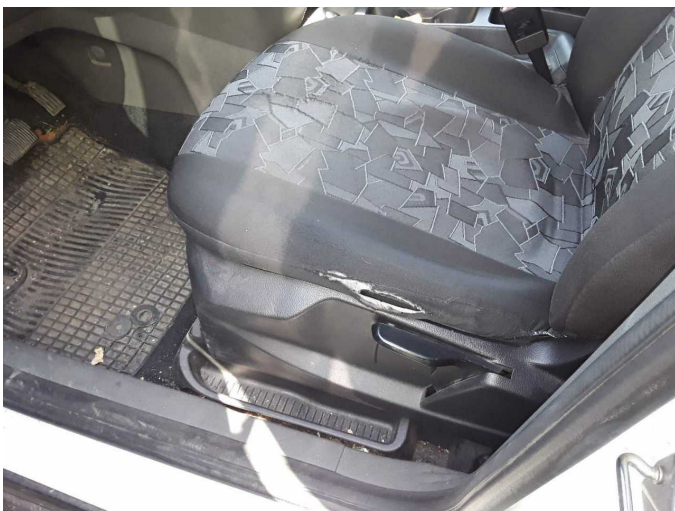
Damage 1: Seat - front: Protective Cover - left side - Broken / torn - Replace
