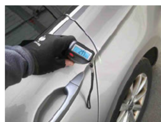
Paint thickness Door RL
