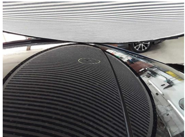
Damage #5: Roof: Roof - dent(s) - Smooth repair work
