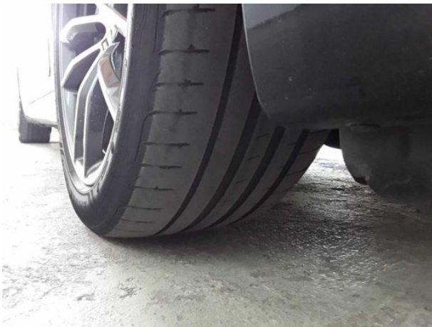
Damage #4: Wheel / tyres: Tyre - front - Worn - Replace
