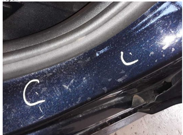
Damage #2: Sill - left side: Sill - Scratched - Smart repair
