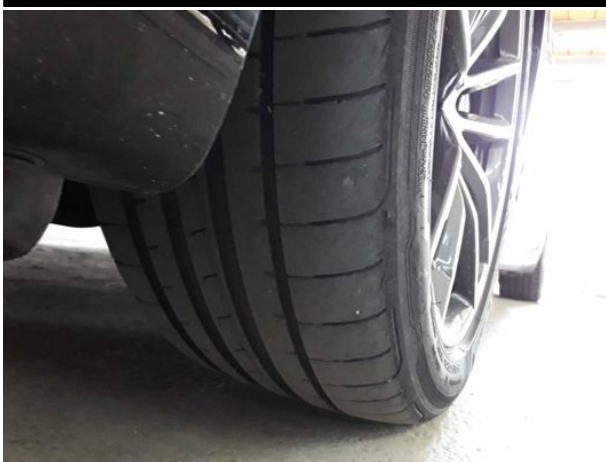
Damage #4: Wheel / tyres: Tyre - front - Worn - Replace
