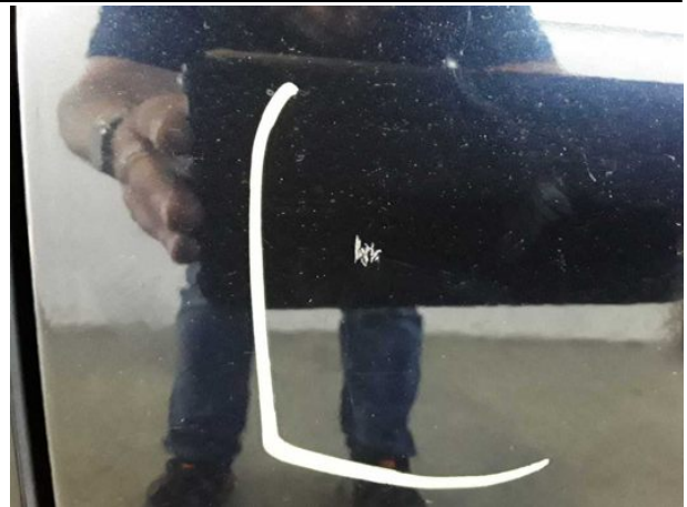
Damage #7: Mudguard - right side: Mudguard - right side - Scratched - Paint
