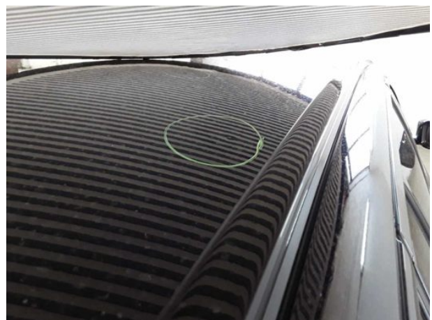
Damage #5: Roof: Roof - dent(s) - Smooth repair work
