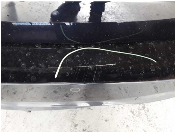
Damage #12: Rear bumper: Rear bumper - Deformed - Replace
