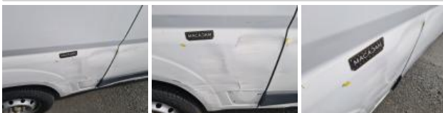
Wing trim RR, Missing, Replace
