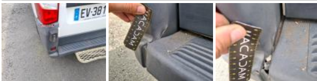
Bumper R, Deformed / Strained, Replace
