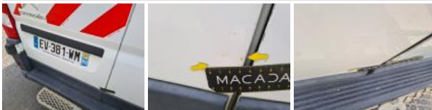
Tailgate lock, Missing, Replace
