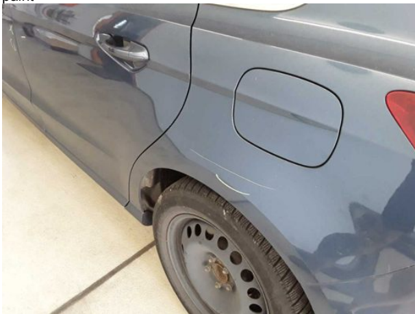
Damage #14: Side panel - rear left side: Side panel - Scratched - Repair and paint
