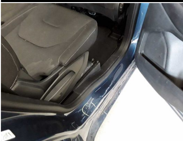
Damage #10: Side panel - rear right side: Sill - Dent / paintcoat damage - Repair and paint
