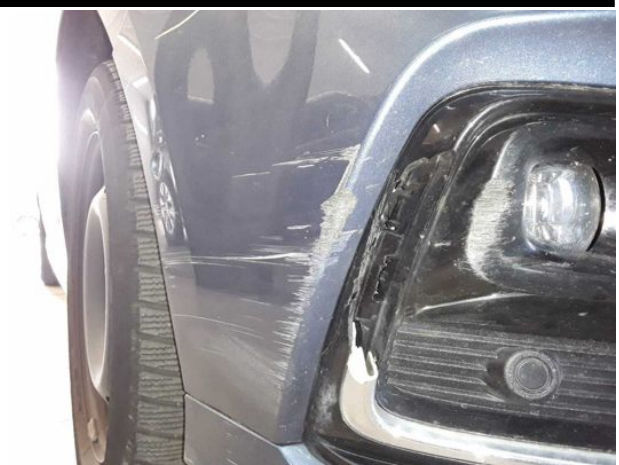
Damage #16: Front bumper: Front bumper - Damaged - Replace
