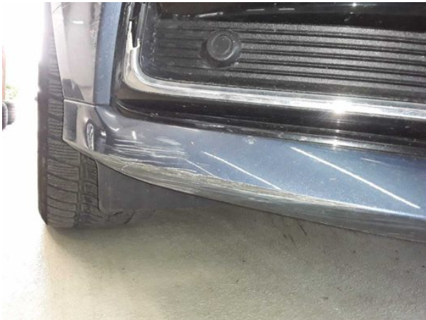
Damage #16: Front bumper: Front bumper - Damaged - Replace
