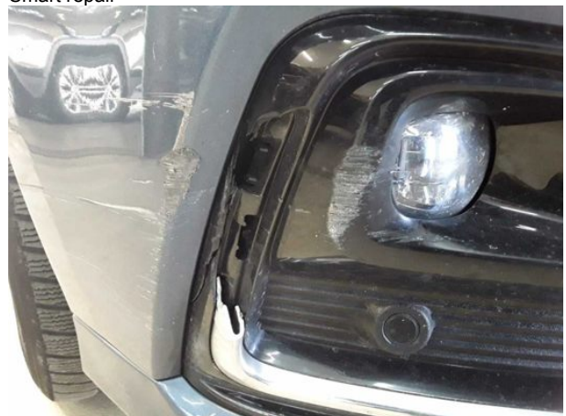
Damage #9: Front bumper: Spoiler - Broken / torn - Replace
