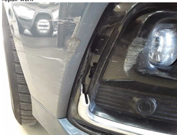
Damage #6: Trim / covers: Trim / covers (Chromleiste) - Broken / torn - Replace
