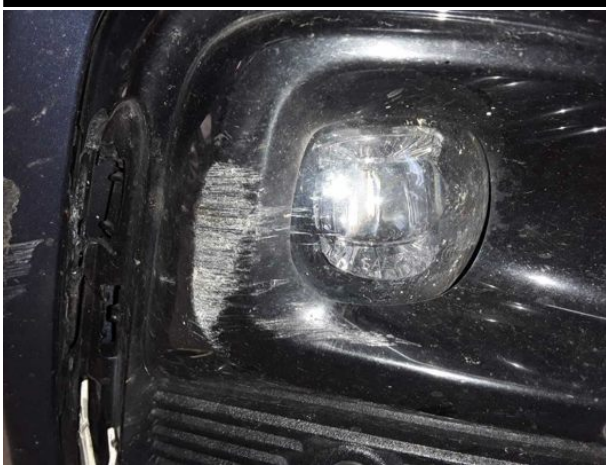
Damage #7: Fog lamp: Fog lamp - front right side - Scratched - Replace
