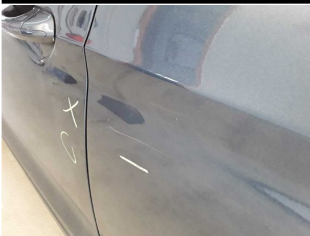
Damage #13: Door - front left side: Door - Scratched - Repair and paint
