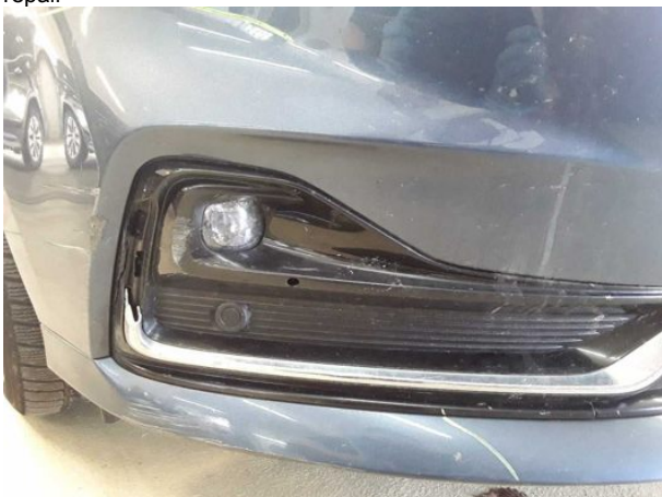
Damage #9: Front bumper: Spoiler - Broken / torn - Replace
