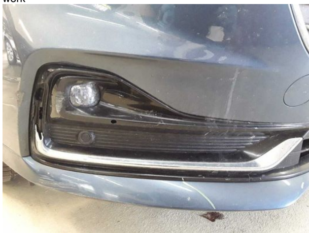
Damage #6: Trim / covers: Trim / covers (Chromleiste) - Broken / torn - Replace
