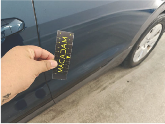
Door RL Scratch(es) Repair and paint (partial) Left
