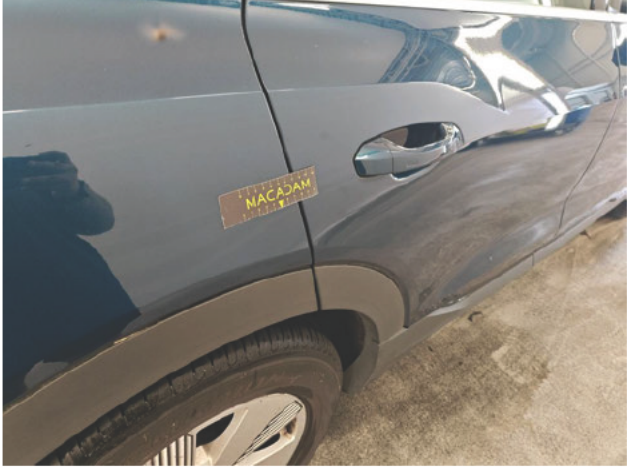
Door RR Scratch(es) Repair and paint (partial) Right
