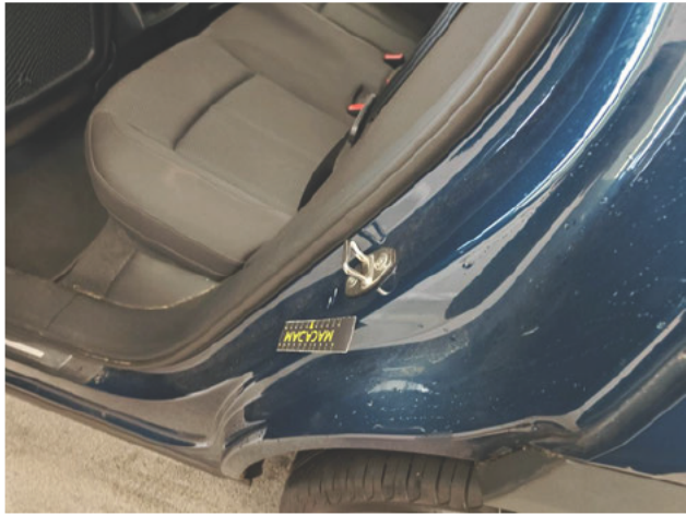
Door frame RL Dent(s) and scratch(es) Repair and paint (complete) Left
