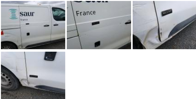
Side wall RR, Dent(s) and scratch(es), Repair and paint (complete)
