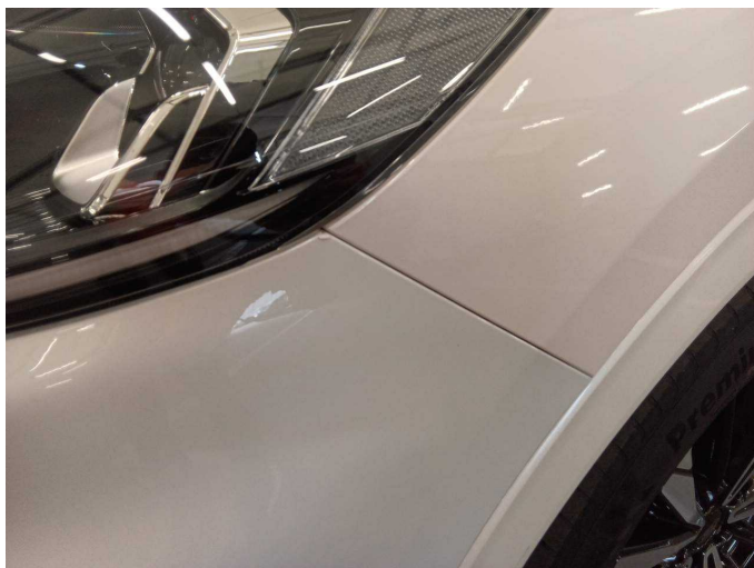
Damage 5: Front bumper: Front bumper (Farbunterschied feststellbar, Anbauteile in Originalfarbe) - Unprofessionally repaired - Paint
