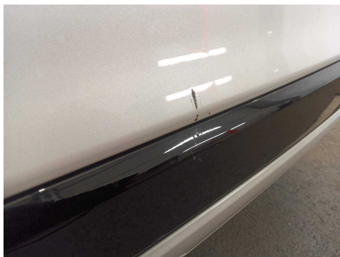
Damage 4: Rear bumper: Rear bumper - Scratch(es) - Paint
