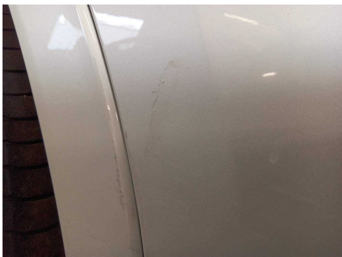
Damage 4: Rear bumper: Rear bumper - Scratch(es) - Paint
