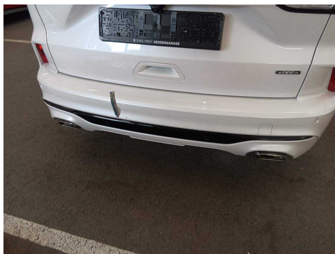
Damage 3: Rear bumper: Protection strip - centre - Scratch(es) - Replace
