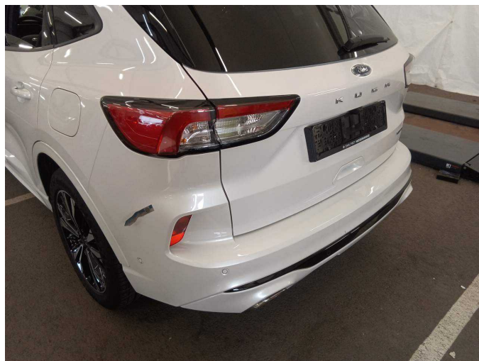
Damage 4: Rear bumper: Rear bumper - Scratch(es) - Paint
