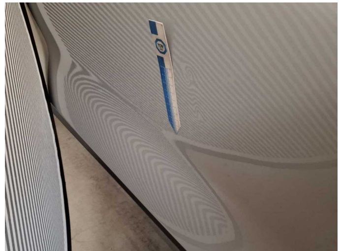
Damage 8: Door - front right side: Door - dent(s) - Smooth repair work
