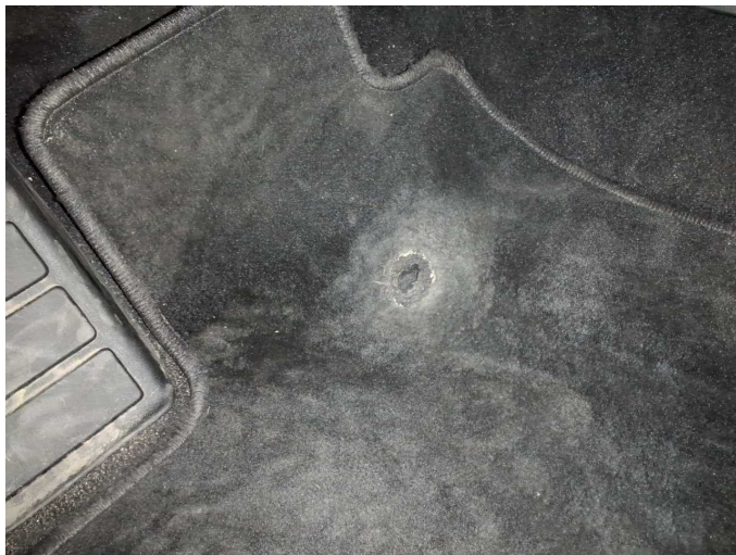
Damage 1: Trim / covers: Floor mats - Holes - Replace
