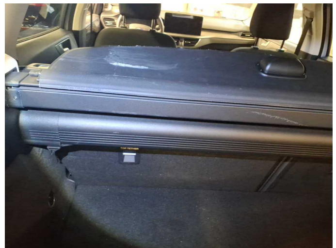
Damage 10: Interior: Boot cover / roller cover - Scratched - Replace
