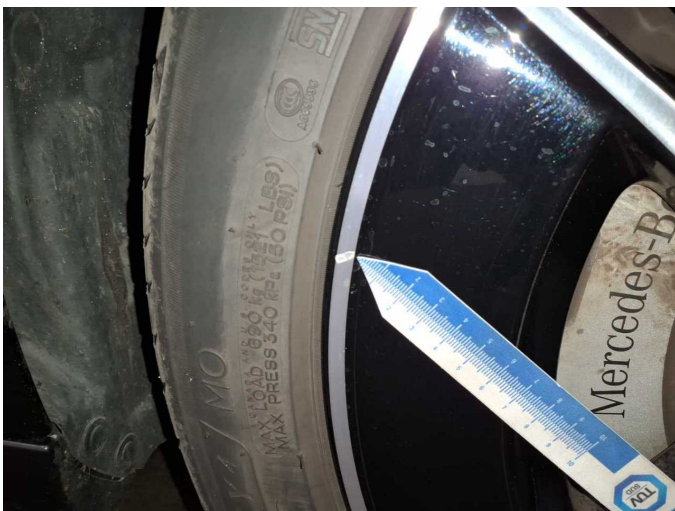
Wear and tear 7: Wheel / tyres: Alloy rim - front right side - Scratch(es) - No deduction
