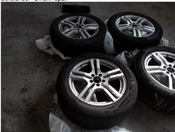
Damage #5: 2nd wheel set: 2 tyres - Worn - Replace
