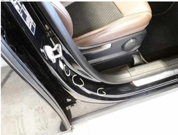
Damage #9: Sill - right side: Sill - Dent / paintcoat damage - Repair and paint
