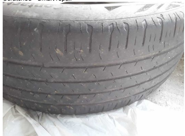
Damage #5: 2nd wheel set: 2 tyres - Worn - Replace
