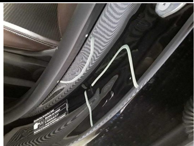
Damage #8: Sill - left side: Sill - Dent / paintcoat damage - Repair and paint
