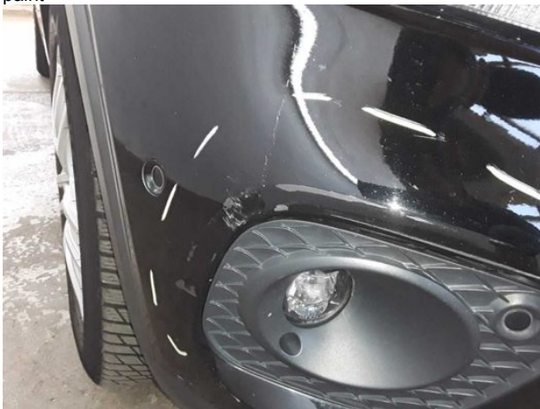
Damage #11: Front bumper: Front bumper - Scratched - Repair a... paint
