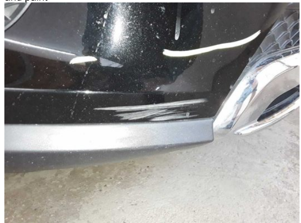
Damage #11: Front bumper: Front bumper - Scratched - Rep... and paint
