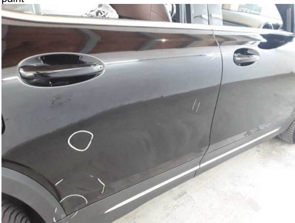
Damage #12: Door - rear right side: Door - Dent / paintcoat dama... - Repair and paint
