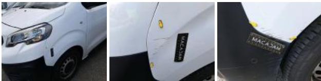
Outer sill L, Dent(s), Replace and paint
