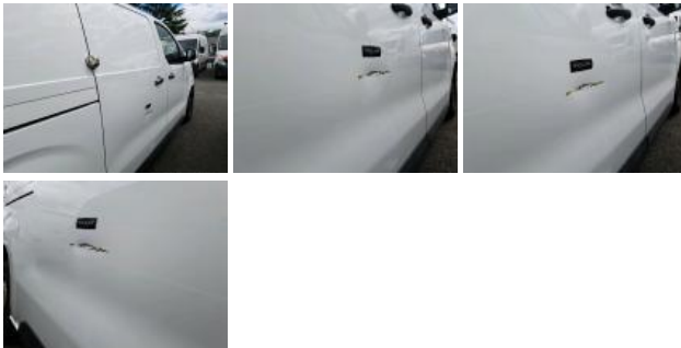
Outer door handle RR, Broken, Replace
