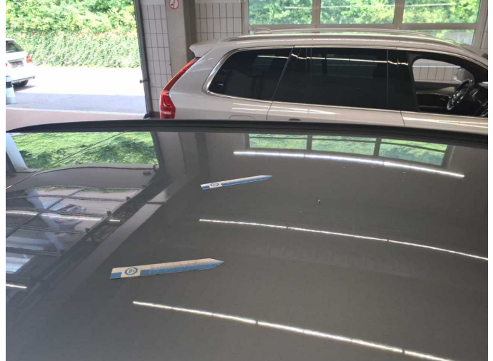
Damage 5: Roof: Roof - dent(s) - Smooth repair work
