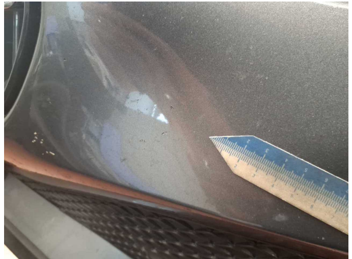
Damage 8: Front bumper: Front bumper - Stone chips - Paint
