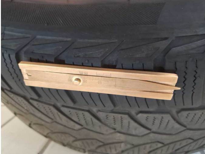
Damage 7: 2nd wheel set: 2 tyres (3mm/ Hinterachse) - Does not meet the leasing specifications - Replace
