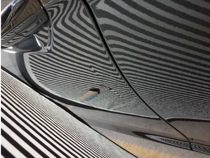
Damage 11: Door - front left side: Door - Deformed - Repair and paint
