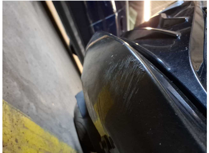
Damage 6: Front bumper: Spoiler - Scratched - Smart repair
