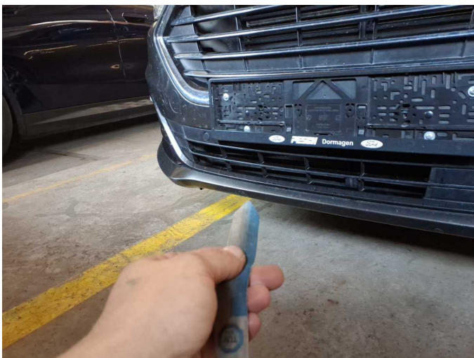
Damage 6: Front bumper: Spoiler - Scratched - Smart repair
