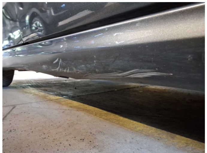
Damage 7: Sill - right side: Trim - Scratched - Paint
