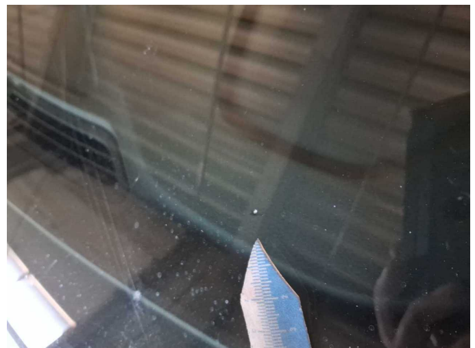
Damage 13: Vehicle glazing: Windscreen (Kein Staubschutz) - Stone chips - repair according to calculation
