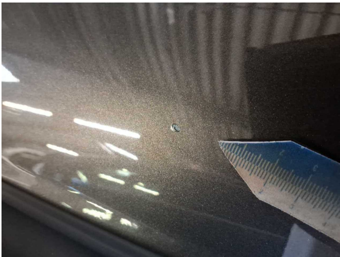
Damage 5: Mudguard - right side: Mudguard - right side - Stone chips - Smart repair
