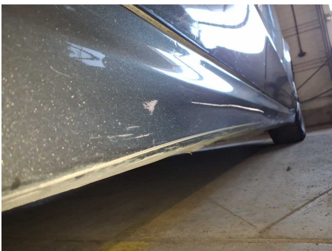
Damage 7: Sill - right side: Trim - Scratched - Paint
