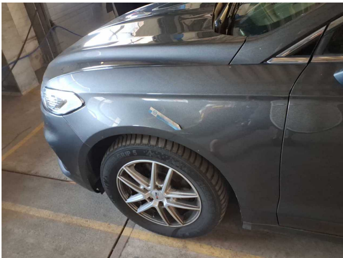
Damage 10: Mudguard - left side: Mudguard - left side - Dent / paintcoat damage - Repair and paint
