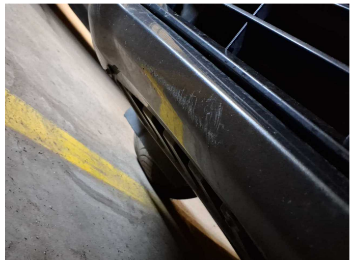
Damage 6: Front bumper: Spoiler - Scratched - Smart repair
