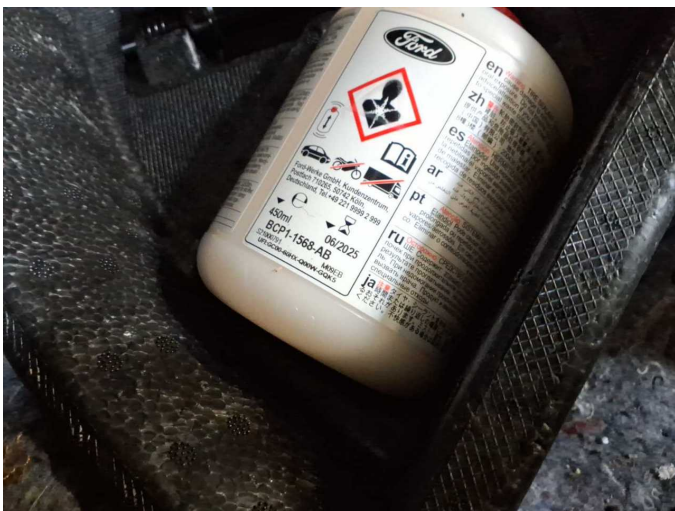
Damage 1: Equipment: Tirefit filler - Expired - Replace
