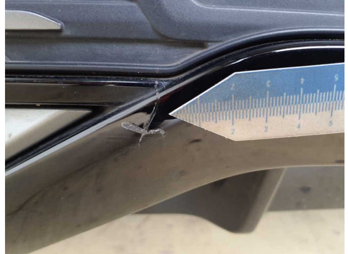
Damage 6: Rear bumper: Spoiler - Scratch(es) - Replace
