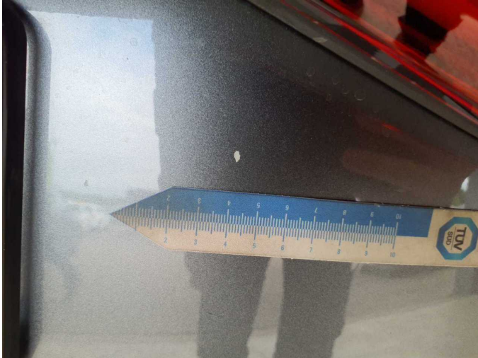
Damage 4: Boot lid / rear door: Boot lid - dent(s) - Smart repair
