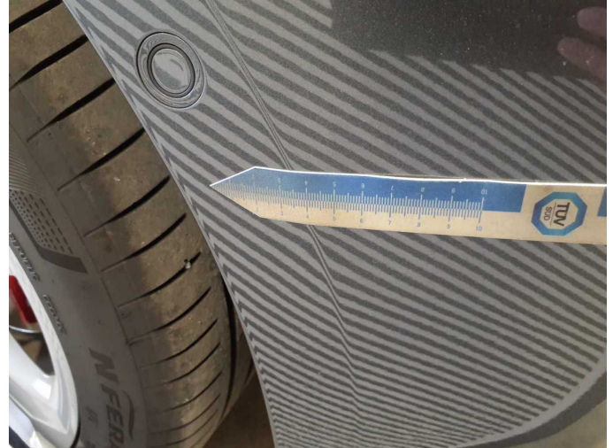
Damage 2: Front bumper: Front bumper - dent(s) - Loss in value
