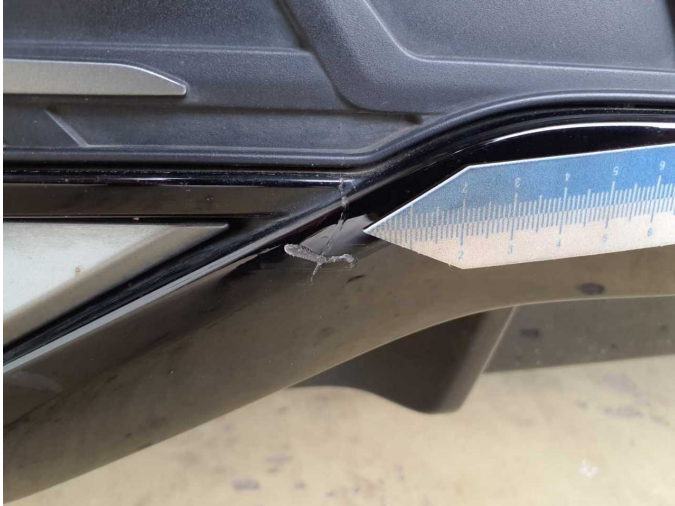
Damage 6: Rear bumper: Spoiler - Scratch(es) - Replace
