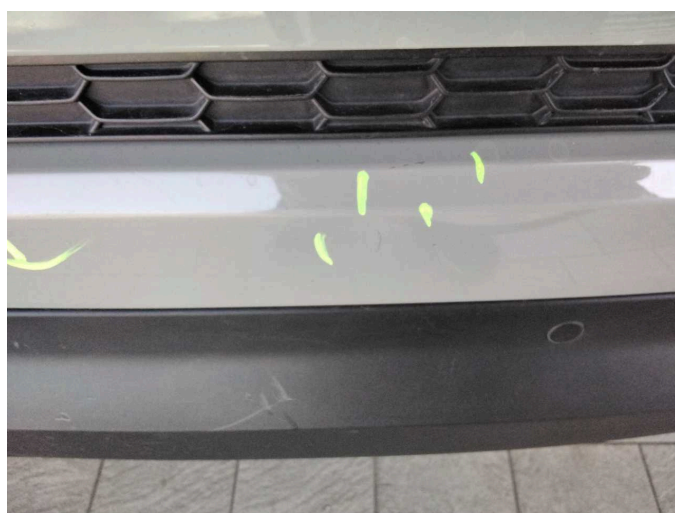
Damage 4: Rear bumper: Rear bumper - Scratch(es) - Smart repair
