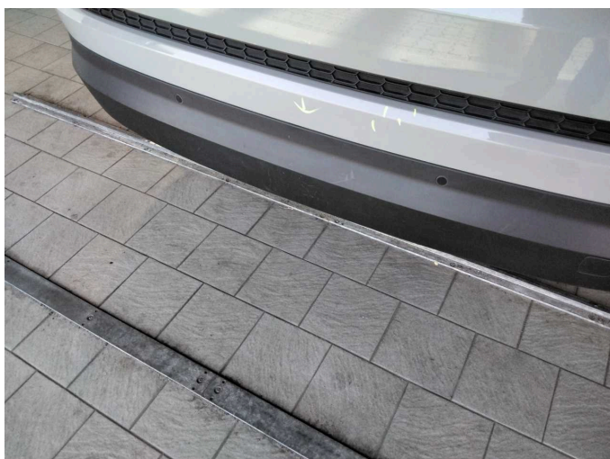
Damage 6: Rear bumper: Spoiler - Scratch(es) - Replace
