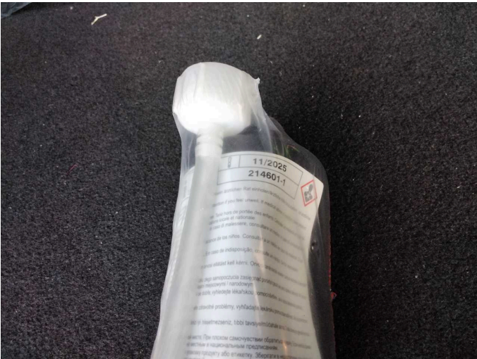
Damage 1: Equipment: Tirefit filler - Expired - Replace
