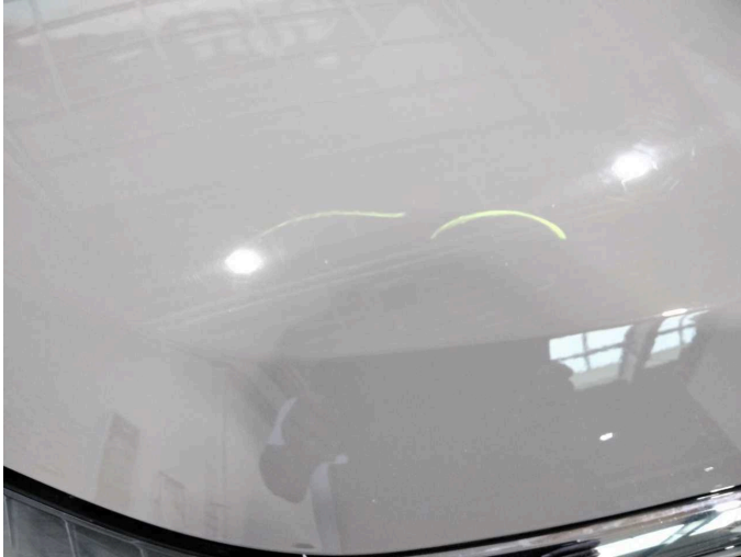
Damage 10: Bonnet: Bonnet - Stone chips - Paint
