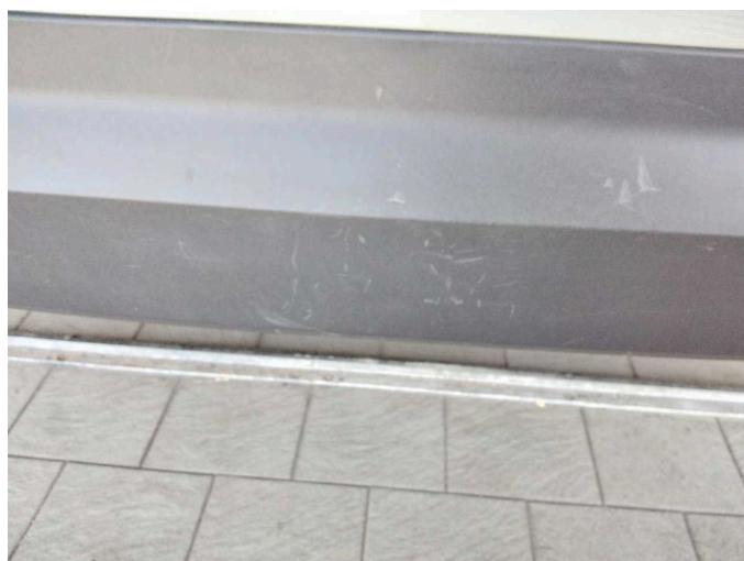
Damage 6: Rear bumper: Spoiler - Scratch(es) - Replace
