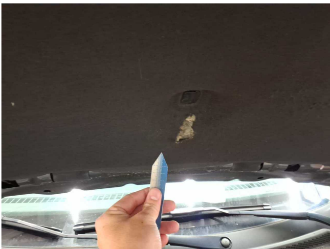
Damage 2: Bonnet: Insulation lining - Broken / torn - Replace
