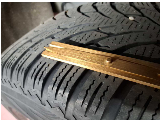
Damage 5: Wheel / tyres: Tyre - right (3mm Profil) - Does not meet the leasing specifications - Replace
