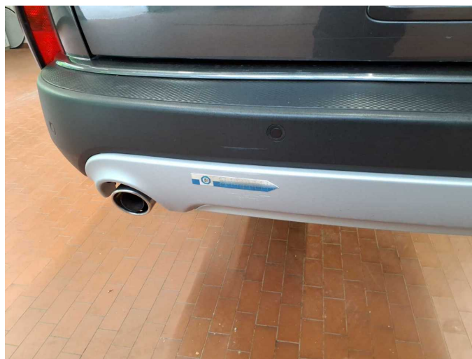
Damage 4: Rear bumper: Spoiler - Scratch(es) - Replace
