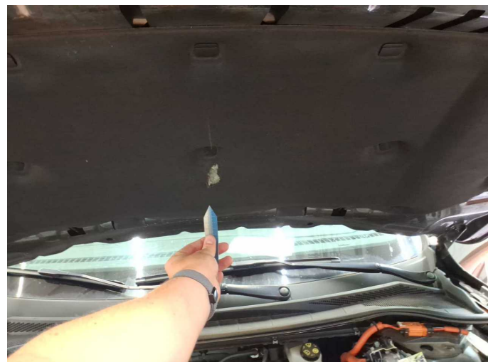
Damage 2: Bonnet: Insulation lining - Broken / torn - Replace
